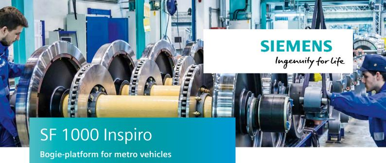
The SF 1000 was designed as a platform bogie for the use in heavy metro vehicles with maximum speeds up to 90 km/h and a maximum axle load of 13.5 t.
