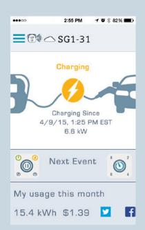
Customers are able to monitor and control the charging status, charging schedule, and power level remotely through the VersiCharge SG SmartPhone App or via provided web pages.
