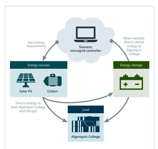
Algonquin College can create, direct and store its own energy. Siemens microgrid controller sets energy requirements from two energy sources – solar and the cogenerator. These sources then direct energy to both the load (Algonquin College) and to the energy storage. And when needed, the Siemens microgrid controller can direct stored energy to Algonquin College.
