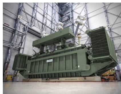
Variable shunt reactor in the test bay.
