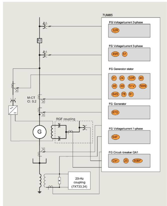
Fig. 6.2-46: High-power generator with protection as sub-packet
