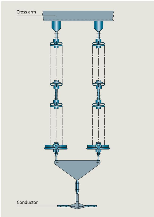
Fig. 2.2-69a: I-shaped suspension insulator set for 245 kV
