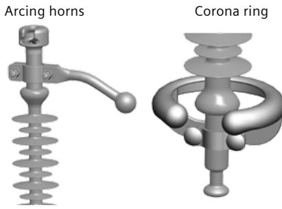
**Recommended corona rings (diameter in mm) by line voltage**
