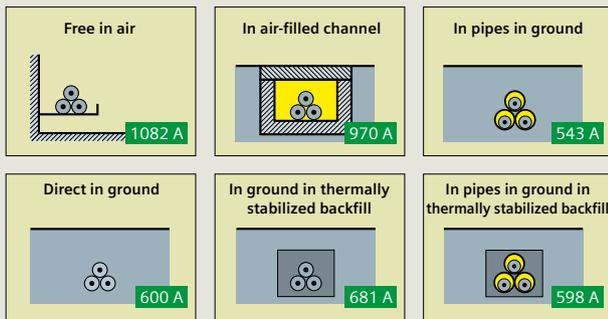
**Conditions:** Cables in trefoil formation, cable screens bonded at both ends, air temperature 30°C, ground temperature 20°C, spec. thermal resistivity of natural 1.0/2.5 km/W, spec. thermal resistivity of thermal stabilized backfill 1.2 km/W, PVC pipes 150 x 5 mm, laying depth 1200 mm, dimensions of cable channel width x height x cover: 1000 x 600 x 150 mm, thermally stabilized backfill in ground 600 x 600 mm, thermally stabilized backfill for pipes 700 x 700 mm
