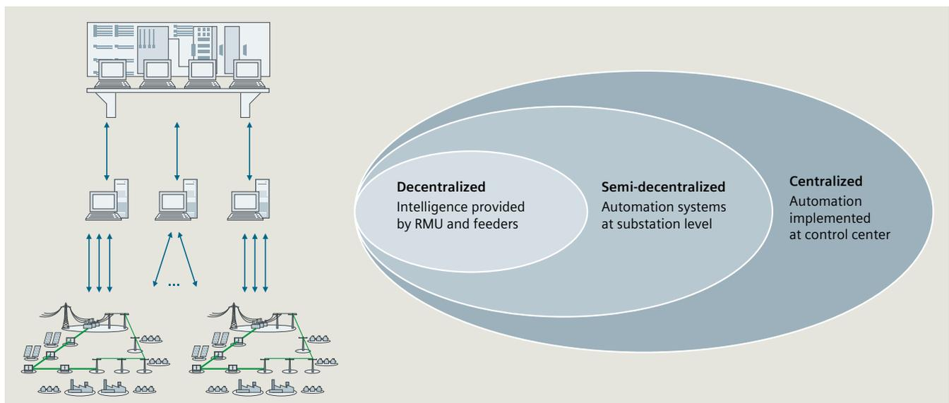
Fig. 6.6-14: Semi-decentralized architecture
