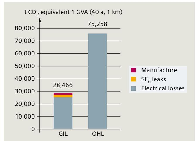
Fig. 2.2-41: Overall CO<sub>2</sub> impact of different transmission systems (one system)
