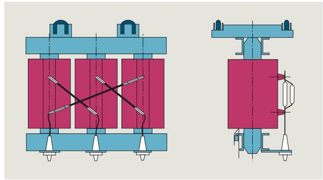
Fig. 5.11-9: GEAFOLE transformer with plug-type cable connections
