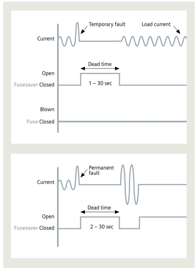
Fig 4.3-15: Modes of operation of the Fusesaver
