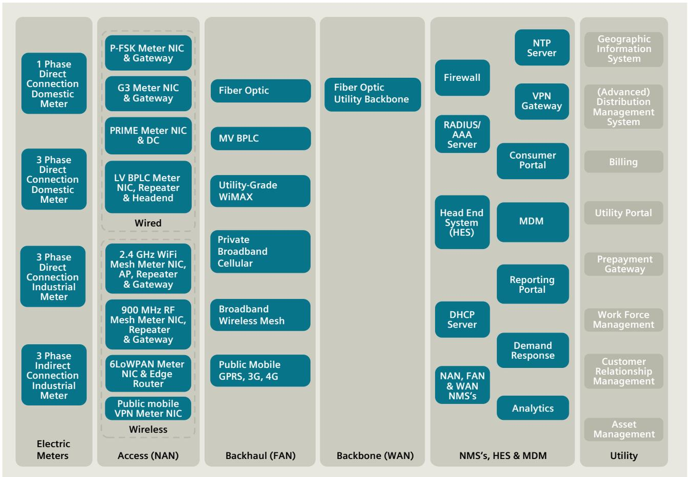
Fig. 8.3-8: Overview of smart metering turnkey solution components
