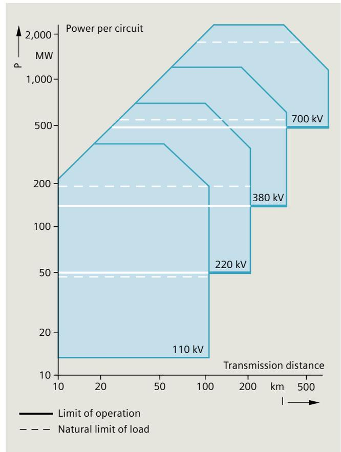
Fig. 2.2-64: Selection of rated voltage for power transmission
