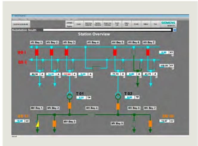
Fig. 6.3-4: Human-machine interface for every control level
