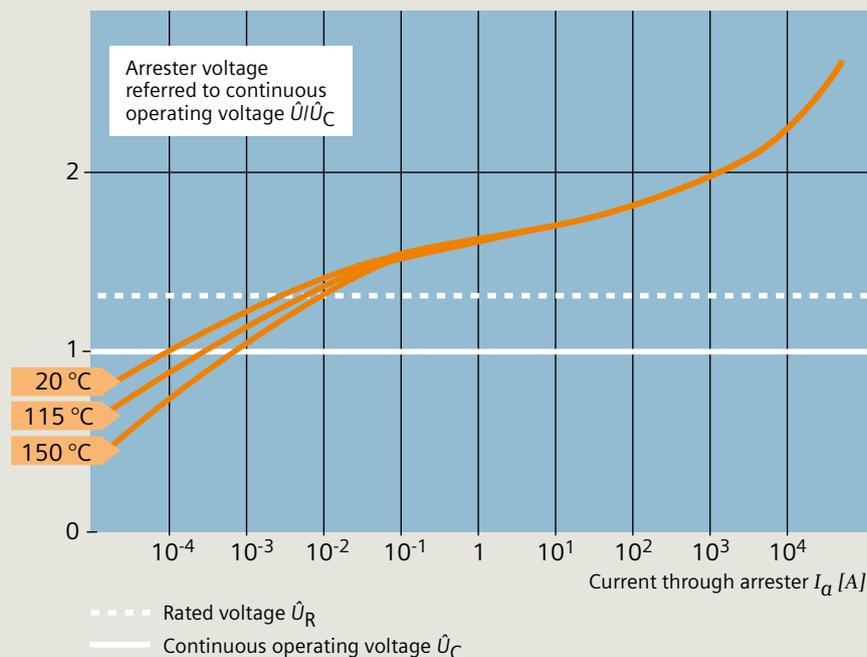
Fig. 4.2-1: Current/voltage characteristics of a non-linear MO arrester
