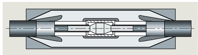
Fig. 2.2-55: Slip-on joint
