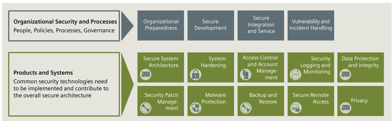
Fig. 2.7-2: Siemens categories of cyber security measures
