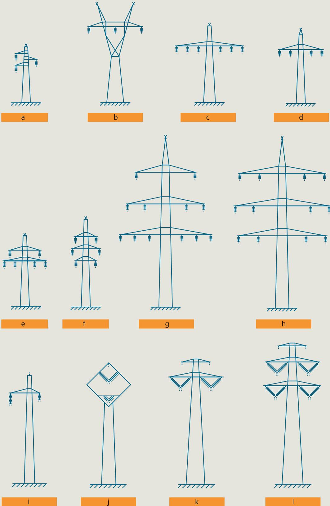
Fig. 2.2-71: (a–h): tower configurations for high-voltage lines (AC); (i–l): tower configurations for high-voltage lines (DC)
