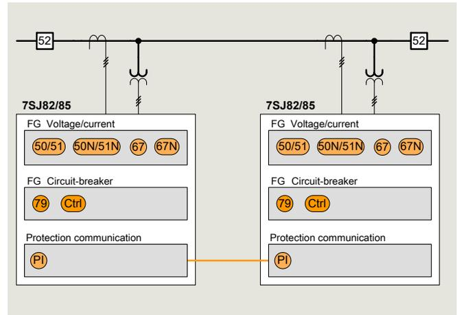
Fig. 6.2-33: Fast fault clearance in double-feed lines (closed) rings
