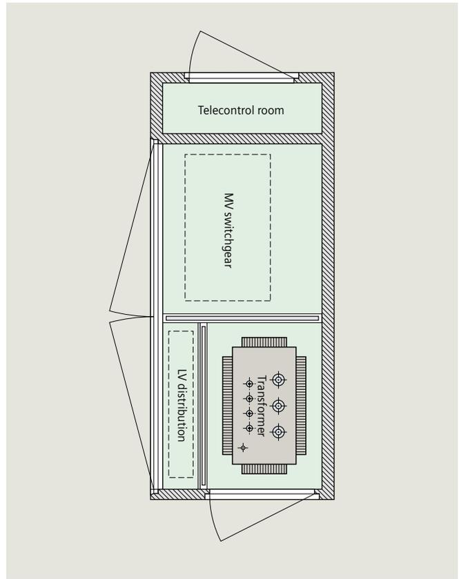
Fig. 2.6-4: Typical room planning of a transformer substation
