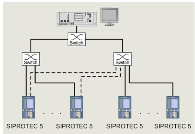
Fig. 6.5-9: Single or redundant connection to external switches
