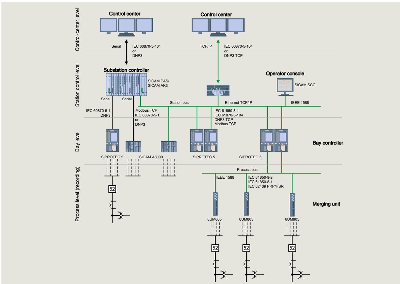
Fig. 6.5-1: Example of protection and substation communication
