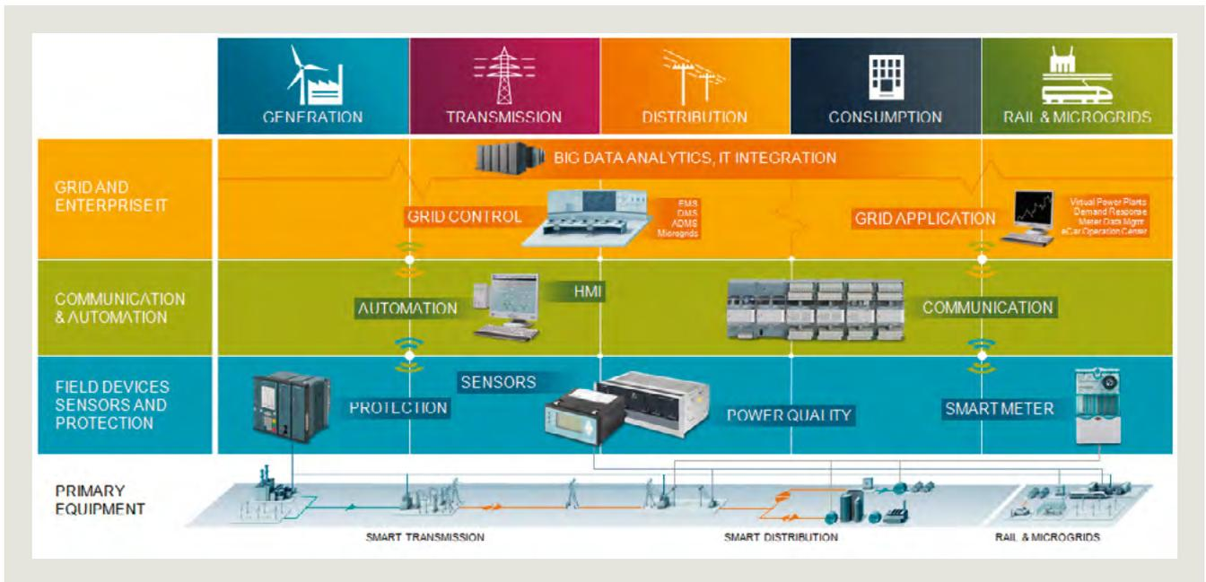
Fig. 7.1-10: Integration on the various process layers
