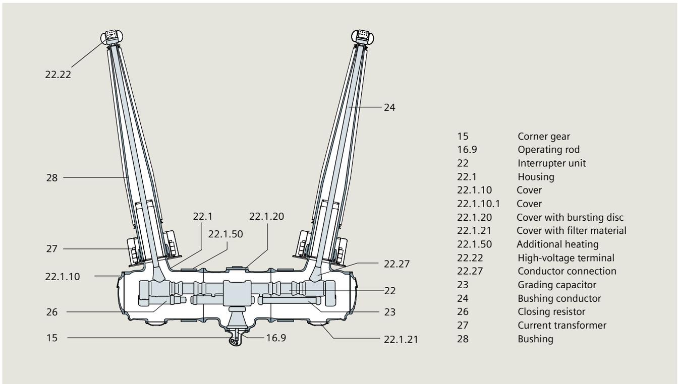
Fig. 4.1-14: Sectional view of a 3AP2/3-DT circuit-breaker pole
