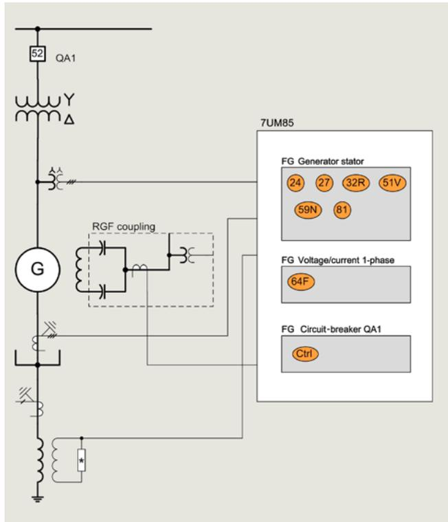
Fig. 6.2-43: Unit connection of a small-power generator
