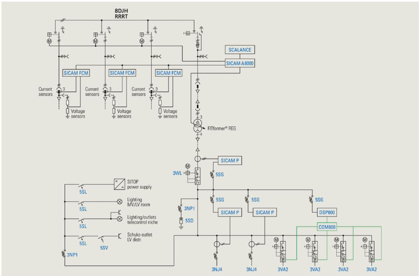
Fig. 2.6-2: Suitable components for an intelligent transformer substation
