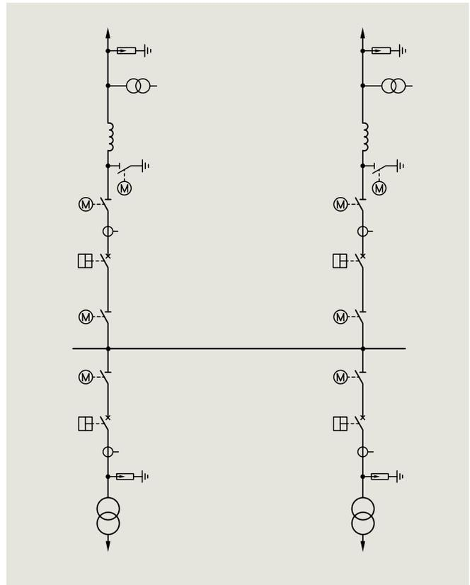
Fig. 3.1-4: Special single busbar, H-scheme (1 BB)
