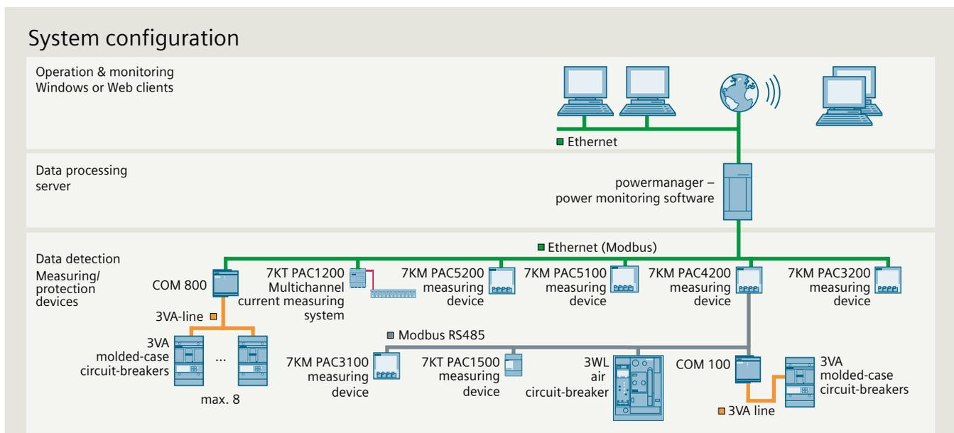
Fig. 4.5-3: Network structure of a power management system
