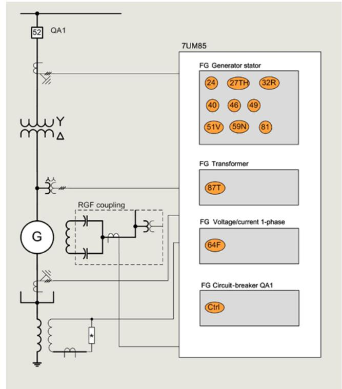
Fig. 6.2-44: Unit connection of a medium-power generator
