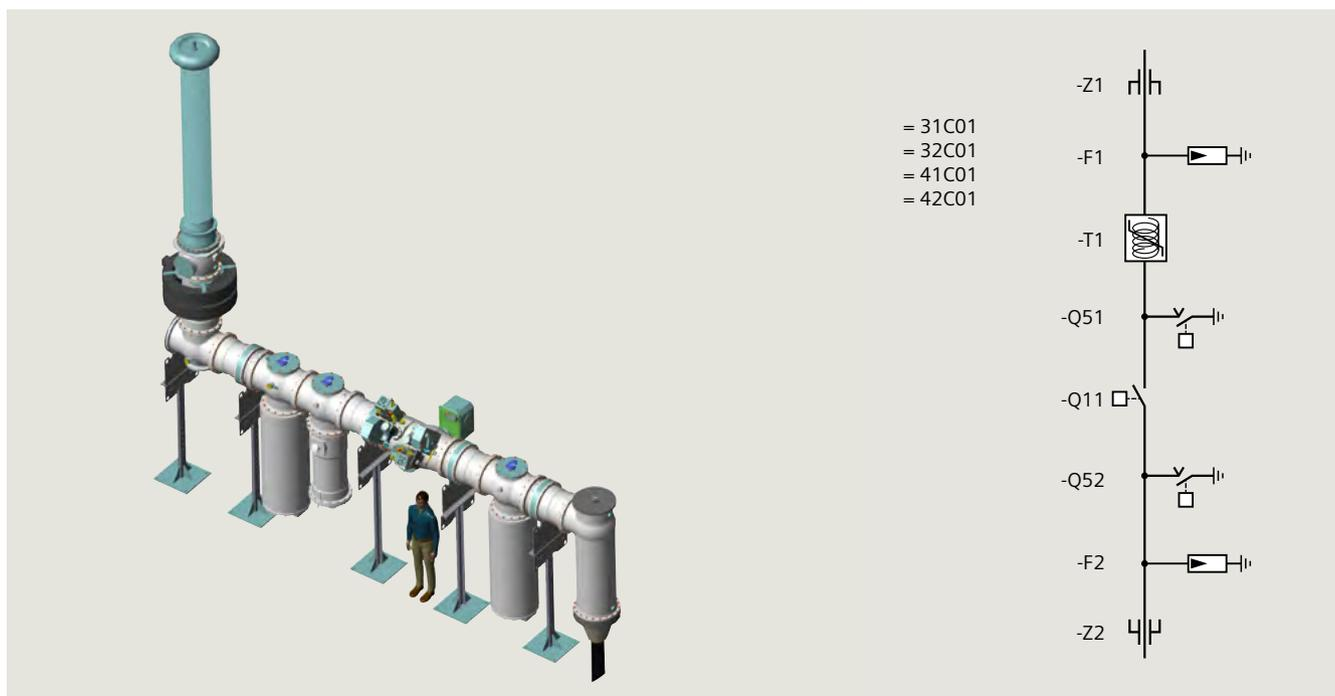
Fig. 2.2-12: 320 kV DC switchyard in/out bay
