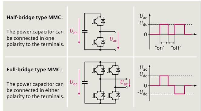
Fig. 2.2-8: MMC topologies: half and full bridge
