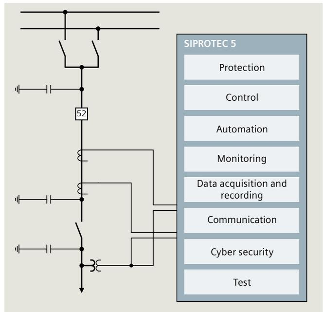
Fig. 6.2-12: Possible functional expansion of SIPROTEC 5 devices
