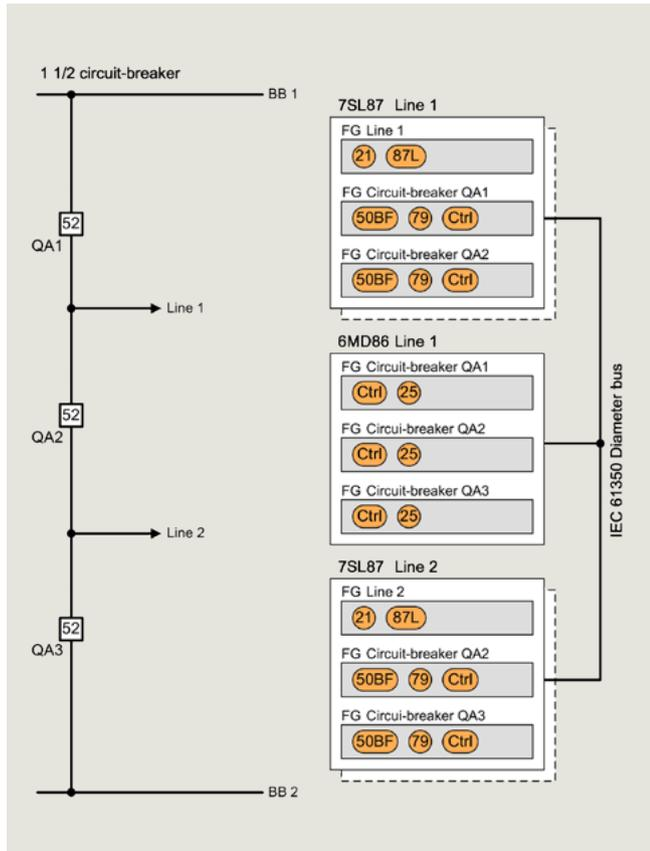
Fig. 6.2-51: Modular and distributed protection and control solution
