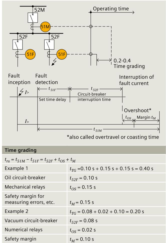
Fig. 6.2-67: Time grading of overcurrent-time relays
