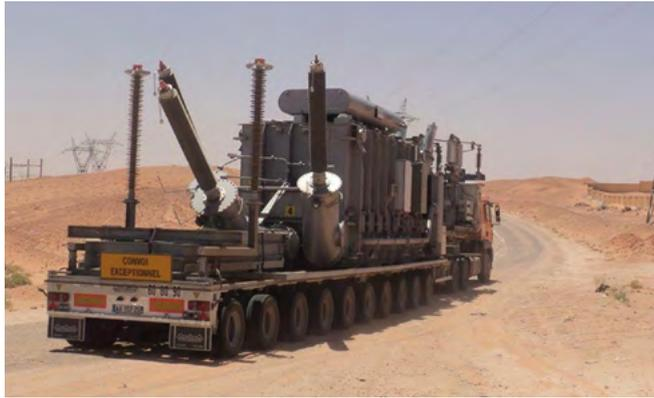
Fig. 2.4-10: 245/60-30 kV 40MVA mobile substation: Transformer trailer
