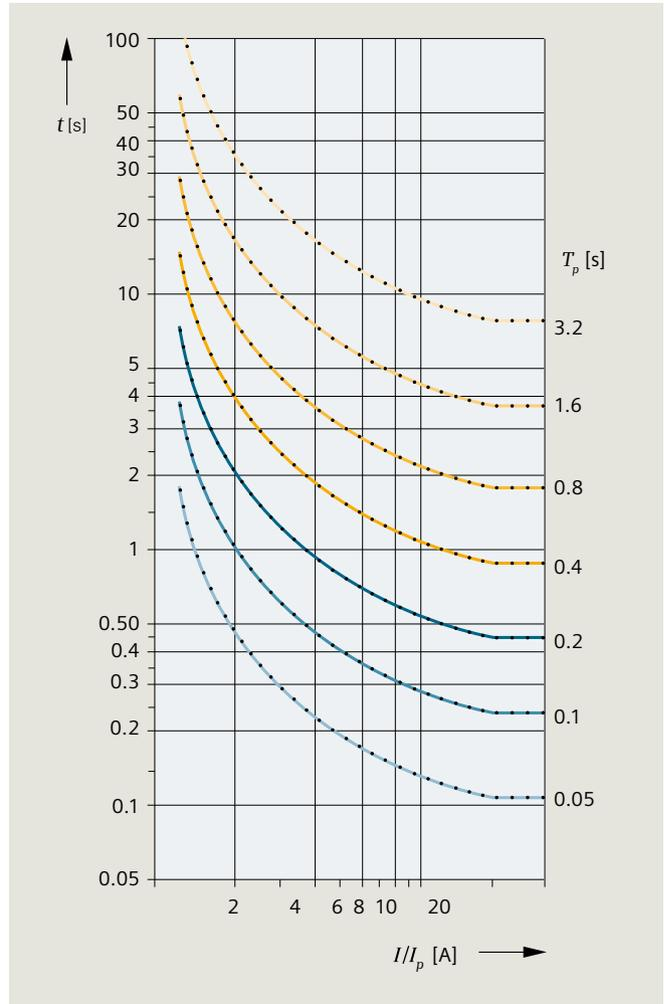
Fig. 6.2-62: Normal inverse-time characteristic of the 7SJ60 relay
