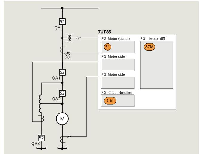
Fig. 6.2-42: Motor differential protection with Korndorfer starter
