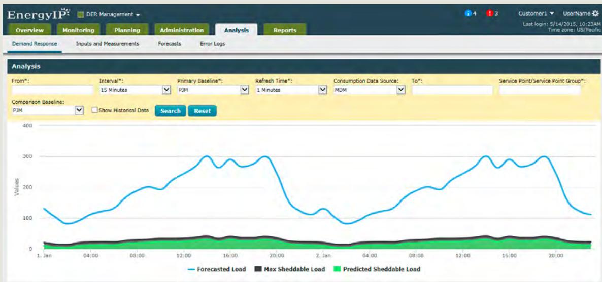
Fig. 7.2-18: EnergyIP user interface for Load Management
