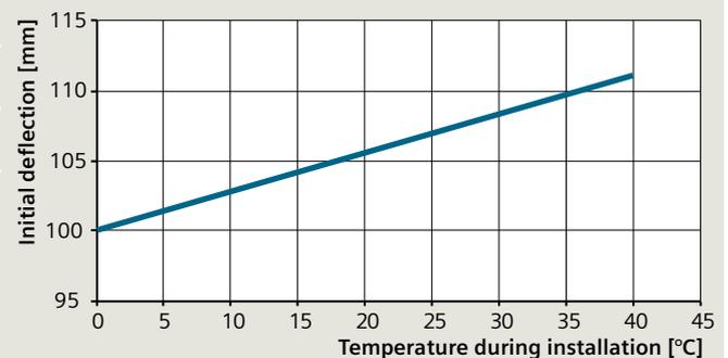
Fig. 2.2-61: Snaking of cables
