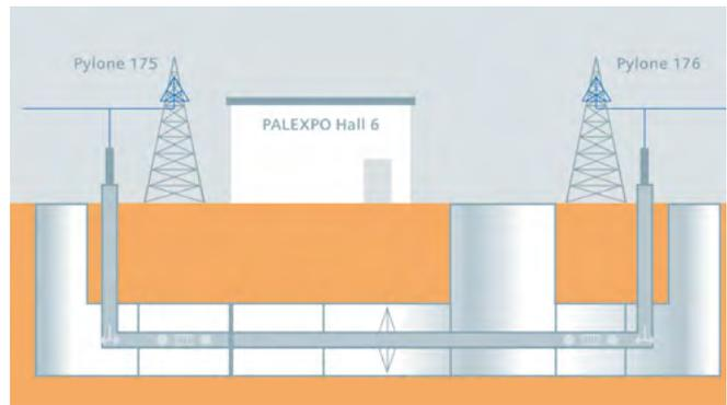
Fig. 2.2-50: GIL replacing overhead line (Palexpo, Geneva, Switzerland)
