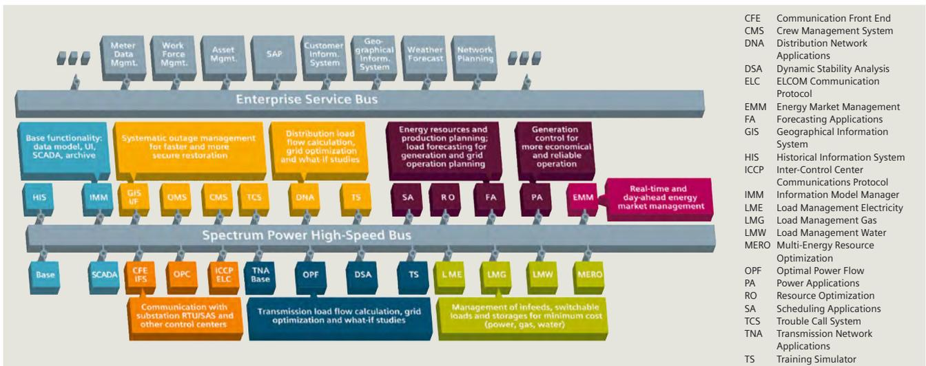
Fig. 7.1-3: Power control system – components overview
