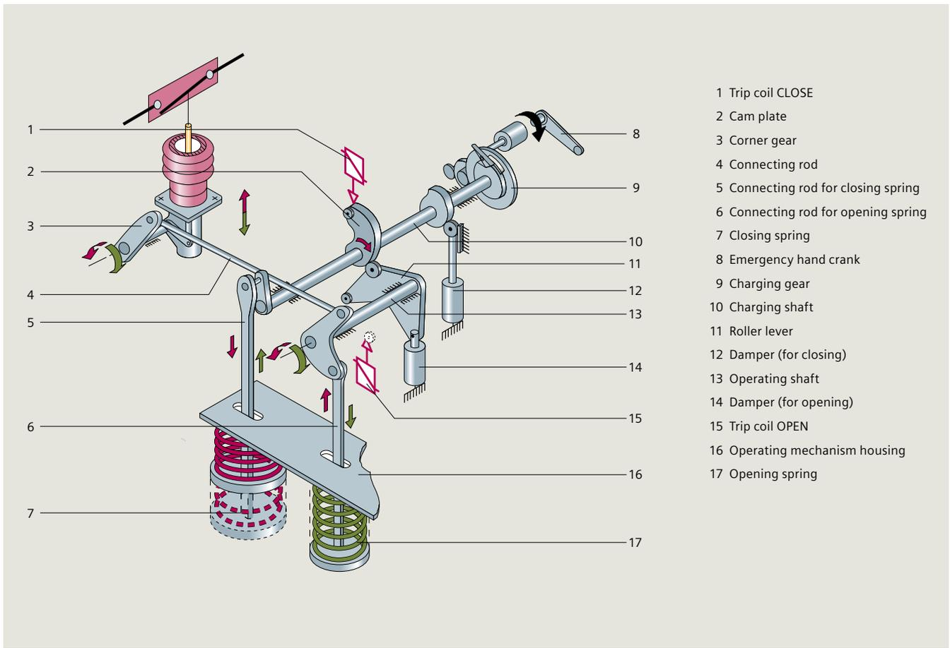
Fig. 4.1-3: Operating mechanism
