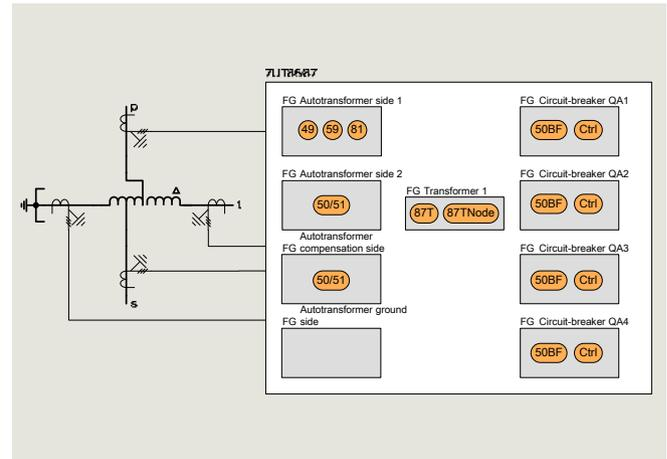
Fig. 6.2-37: Autotransformer bank
