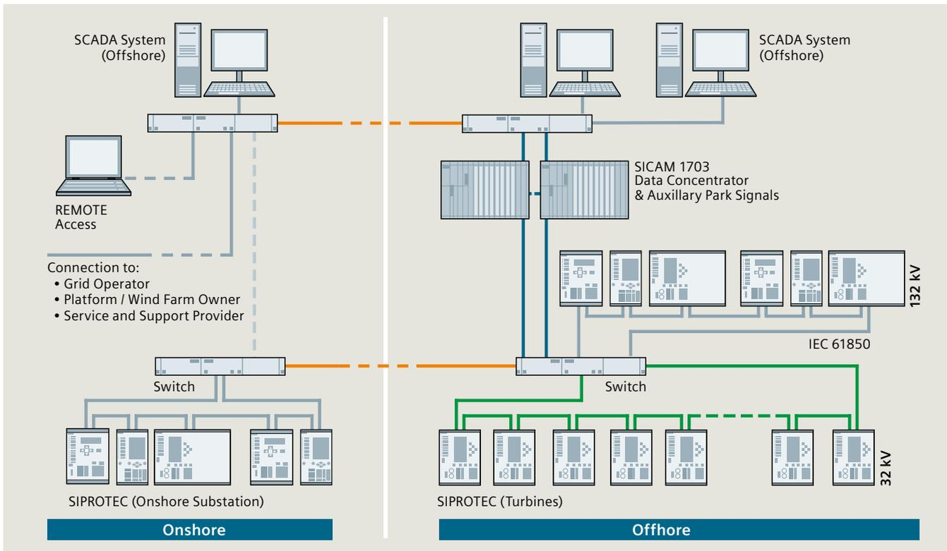
Fig. 6.6-26: SCADA system with onshore and offshore part
