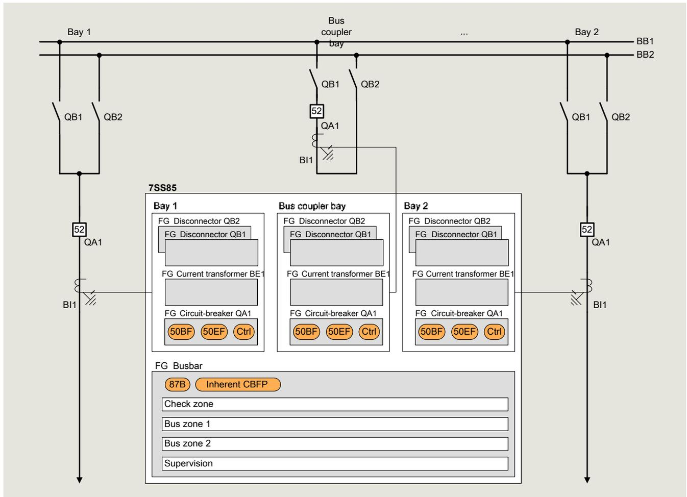
Fig. 6.2-55: Double busbar feeder with busbar coupler
