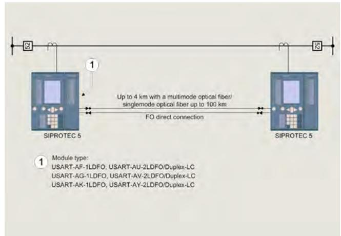
Fig. 6.5-21: Protection communication via direct optical fiber
