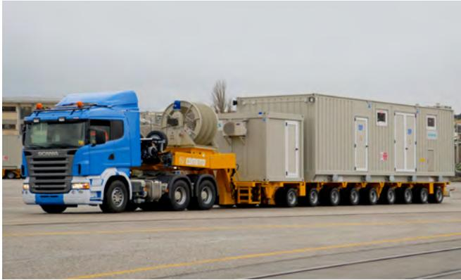
Fig. 2.4-12: 36kV/12kV 16 MVA mobile substation
