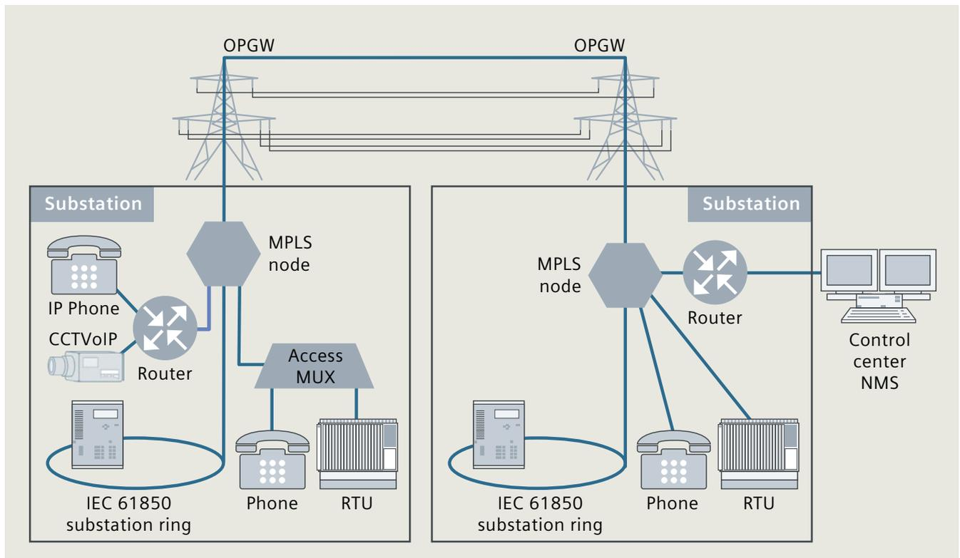
Fig. 8.1-2: MPLS communication solution for transmission grids
