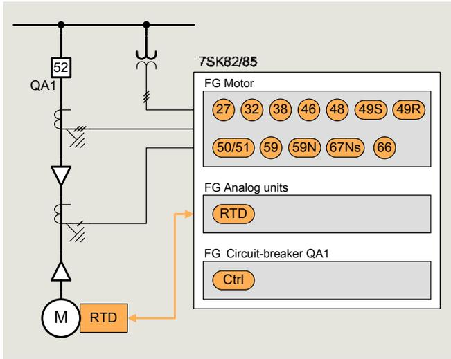
Fig. 6.2-39: Protection and control for induction motor
