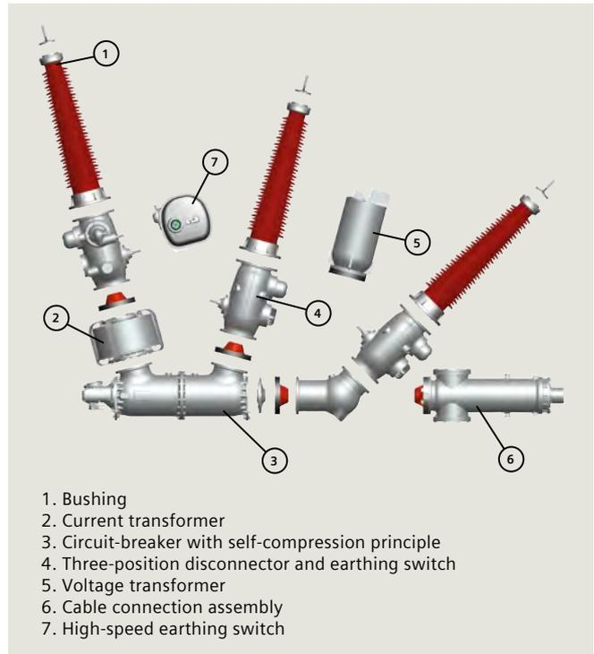
Fig. 4.1-16: Possible components for the 3AP1 DTC
