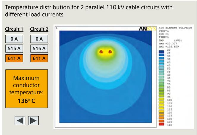
Fig. 2.2-59: Temperature distribution for 2 parallel 110 kV cable circuits
