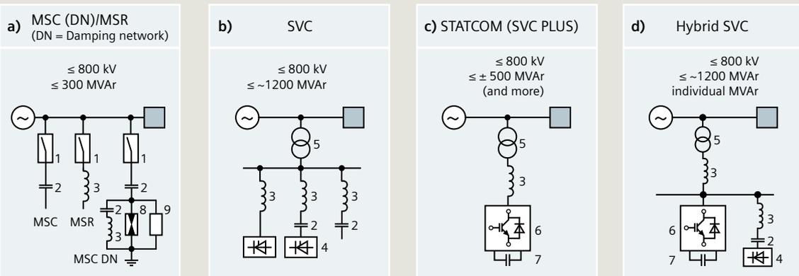
1 Switchgear 2 Capacitor 3 Reactor 4 Thyristor valve(s) 5 Transformer 6 IGBT converter 7 DC capacitors 8 Arrester 9 Resistor
