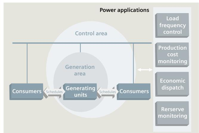
Fig. 7.1-29: Automatic generation control with power applications
