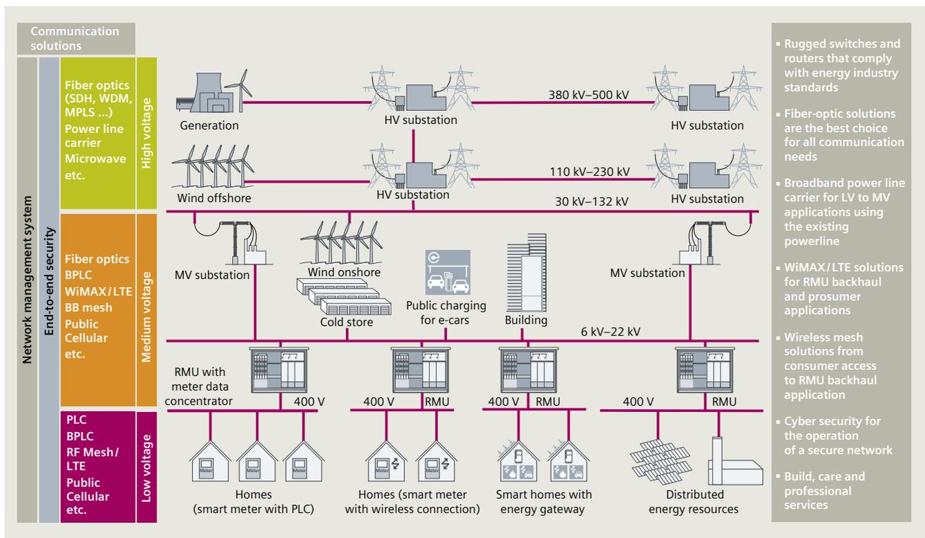
Fig. 8.0-2: Communication network solutions for Smart Grids
