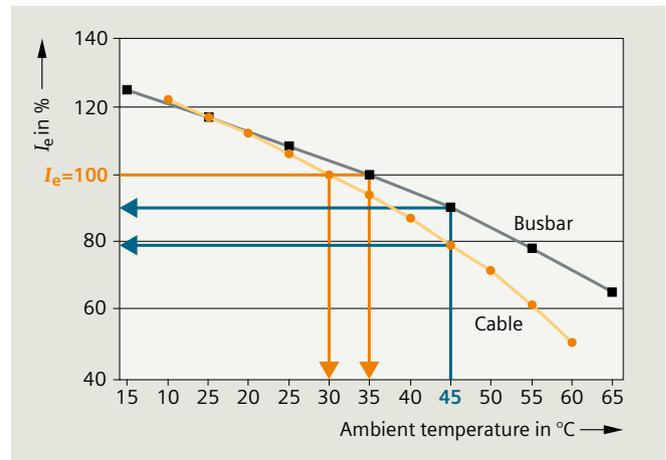
Fig. 3.3-18: Comparison of temperature response and derating
