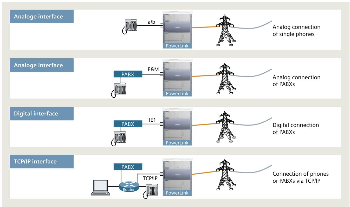
Fig. 8.1-8: Basic options of voice communication via PowerLink
