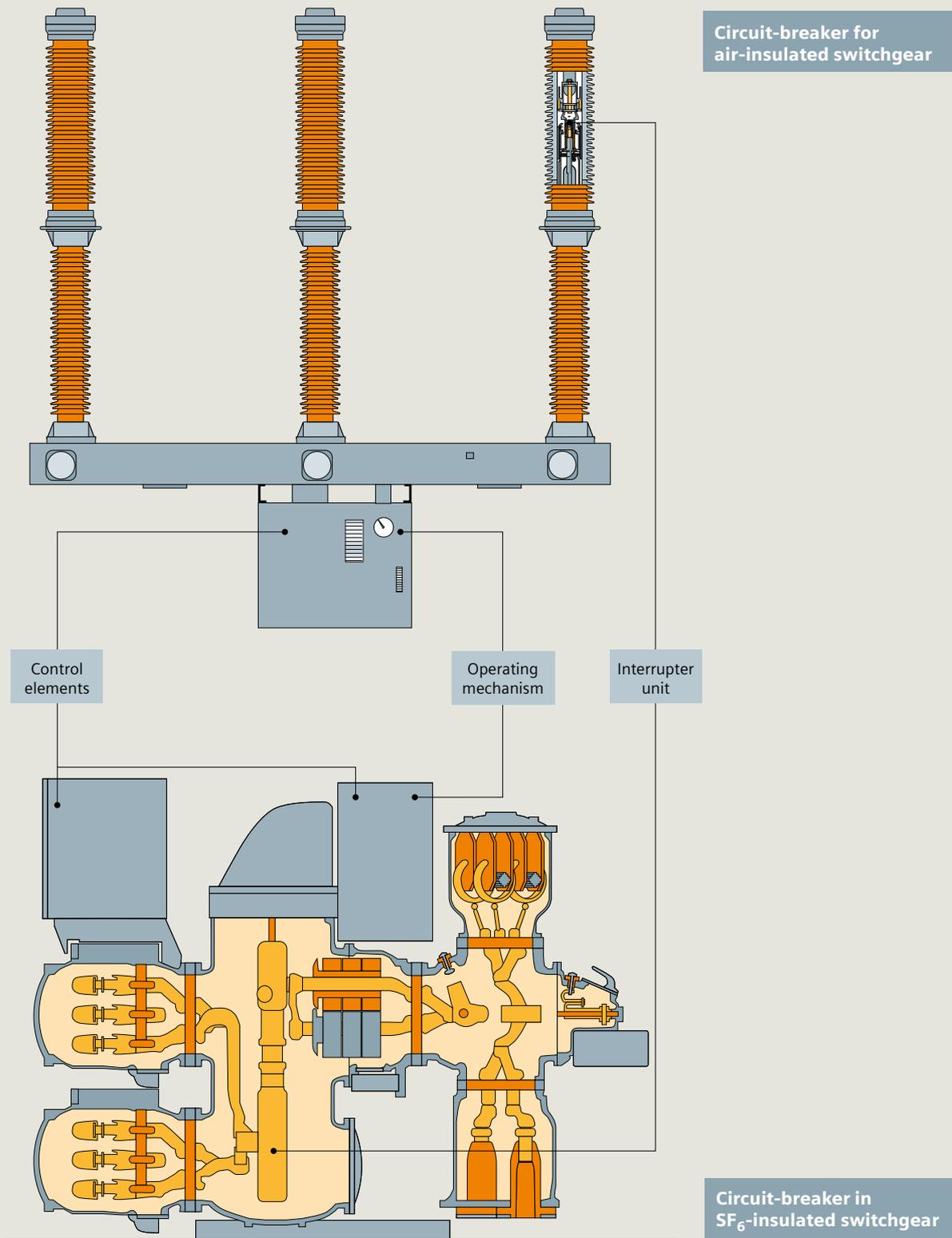
Fig. 4.1-1: Circuit-breaker parts: circuit-breaker for air-insulated switchgear (top), circuit-breaker in SF<sub>6</sub>-insulated switchgear (bottom)
