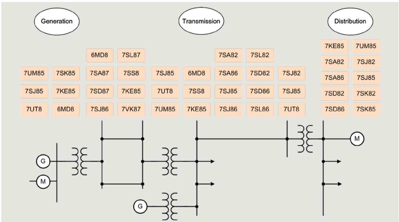
Fig. 6.2-28: Available device types of the SIPROTEC 5 system
