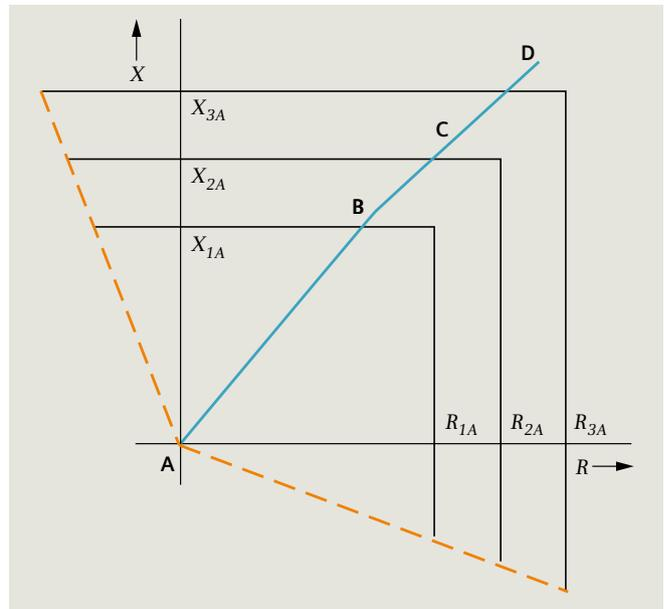
Fig. 6.2-57: Operating characteristics of Siemens distance relays
