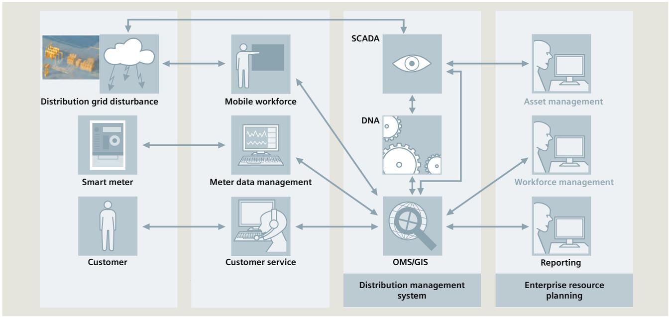
Fig. 7.1-6: Schematic workflow in a distribution management system
