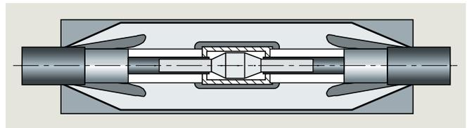
Fig. 2.2-55: Slip-on joint
