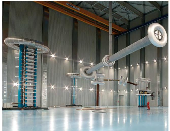
Fig. 4.2-47: Wall bushing – 800 kV HVDC – project Yunnan-Guangdong, China
