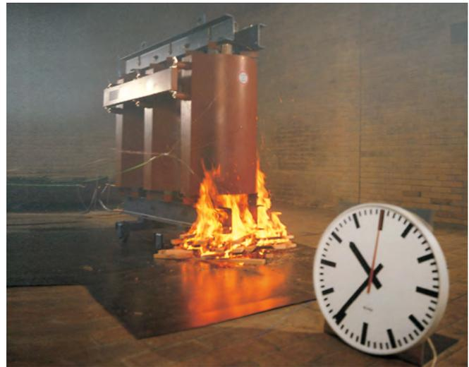
Fig. 5.11-7: Flammability test of cast-resin transformer
