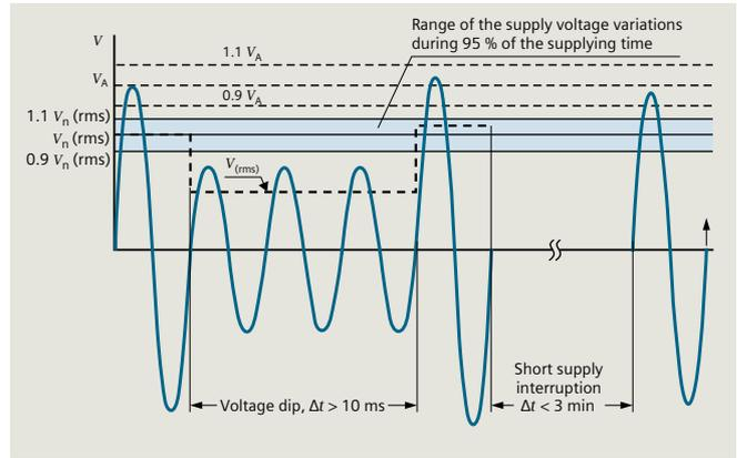
Fig. 6.4-4: Illustration of a voltage dip and a short supply interruption, classified according to EN 50160;  $V_N$  – nominal voltage of the supply system (r.m.s.),  $V_A$  – amplitude of the supply voltage,  $V_{(r.m.s.)}$  – the actual r.m.s. value of the supply voltage
