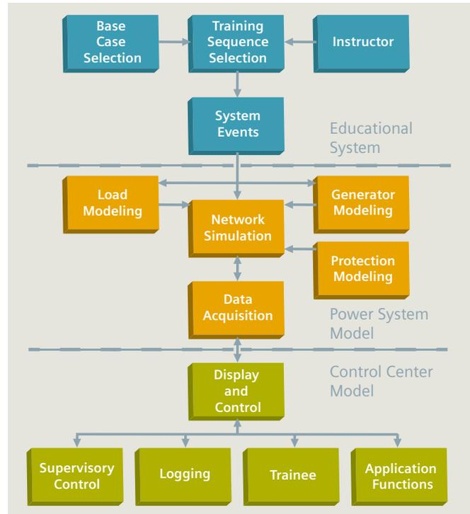
Fig. 7.1-8: Block diagram of a training simulator
