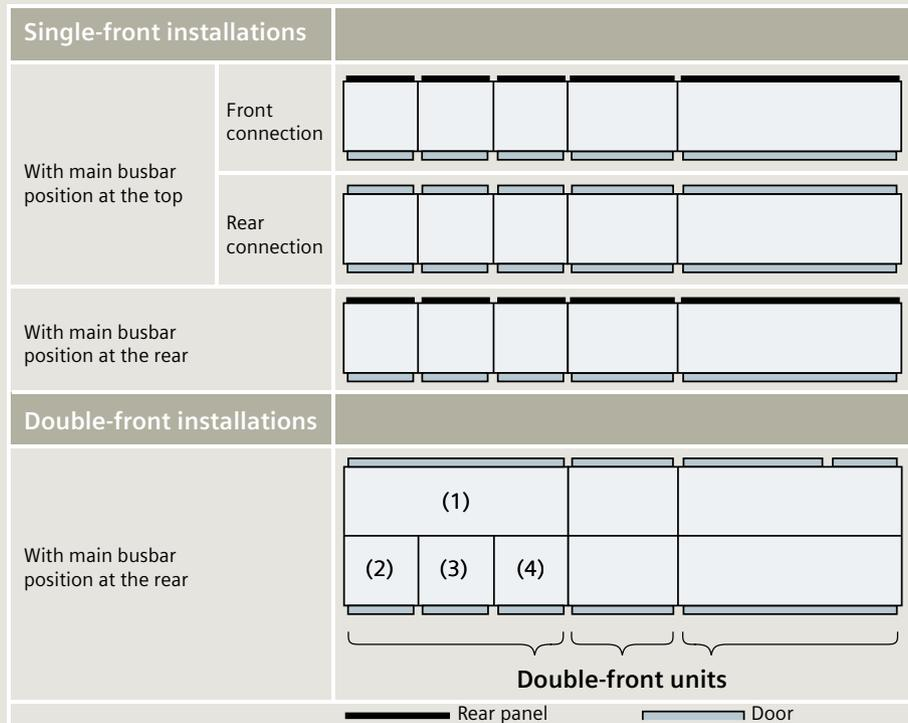
Fig. 3.3-14: Cubicle arrangement for single-front (top) and double-front systems (bottom)
