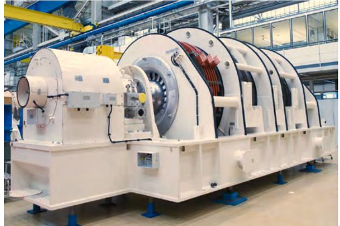
Fig. 2.2-24: Synchronous generator
