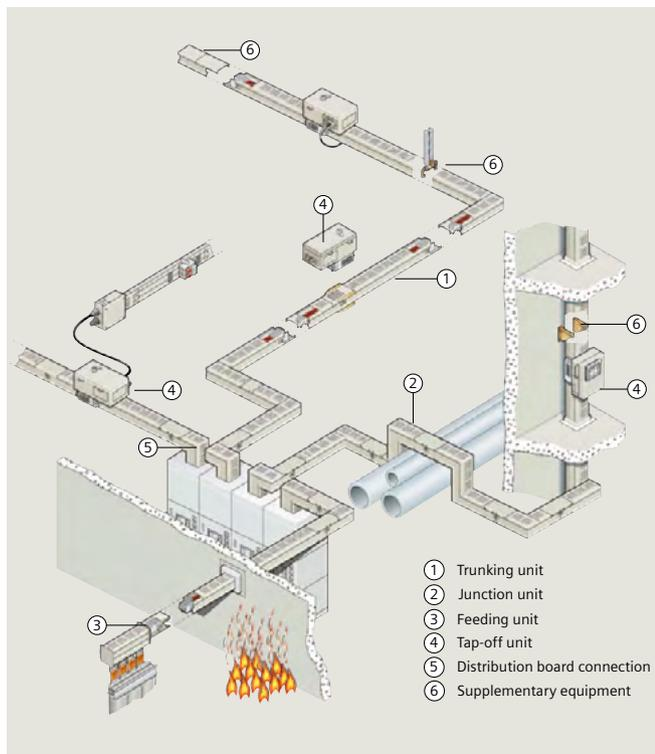
Fig. 3.3-21: System components for LDA/LDC system
