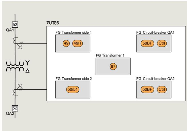
Fig. 6.2-35: Two-winding transformer
