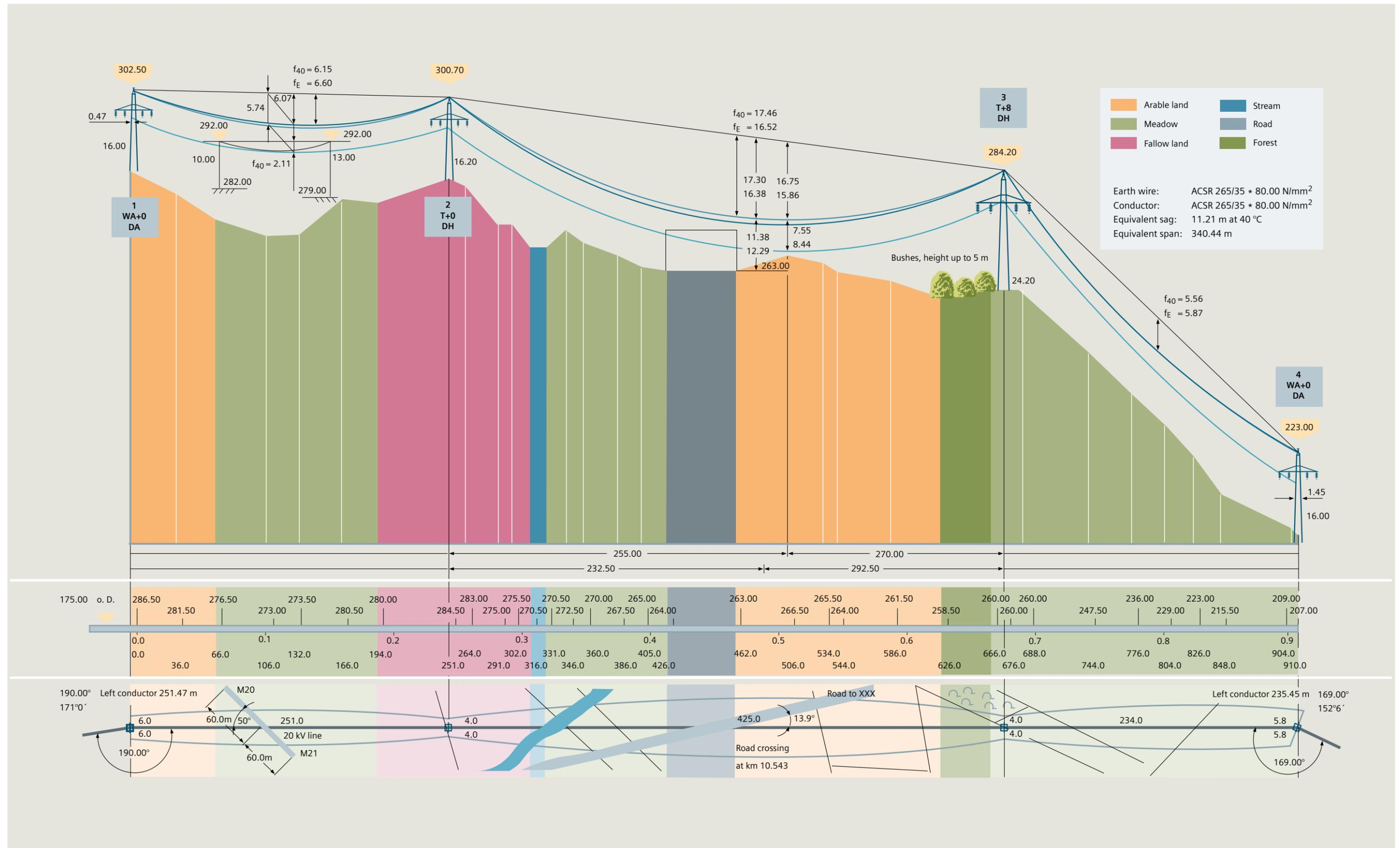
Fig. 2.2-74: Line profile established by computer
