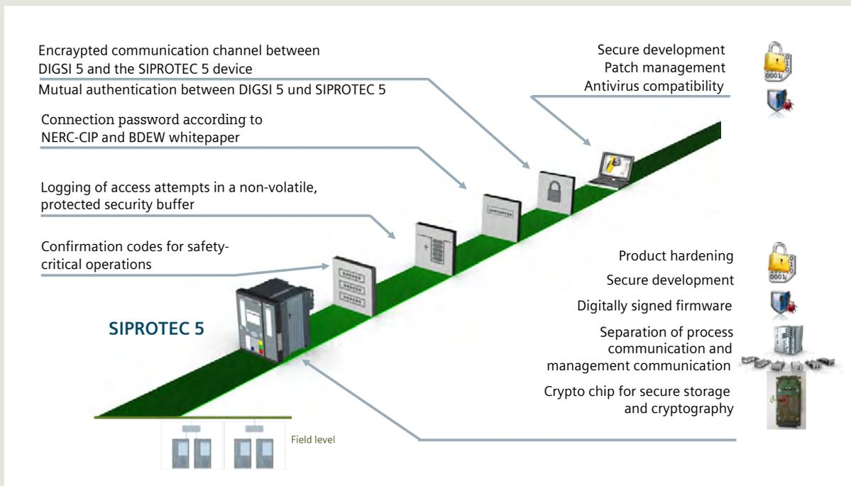
Fig. 2.7-8: Security features of a state-of-the-art protection device
