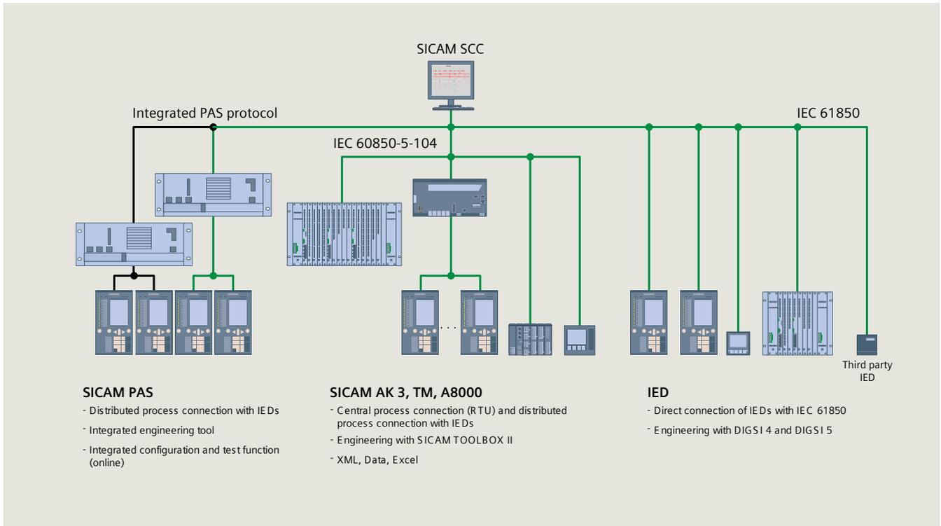
Fig. 6.3-8: Flexible configuration
