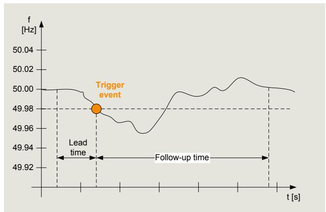
Fig. 6.4-35: Automatic time trigger (example for frequency)
