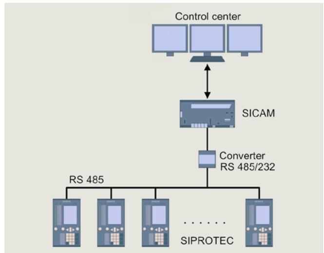
Fig. 6.5-7: Serial bus wiring in accordance with RS 485
