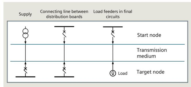
Fig. 3.3-3: Schematic representation of the different circuit types
