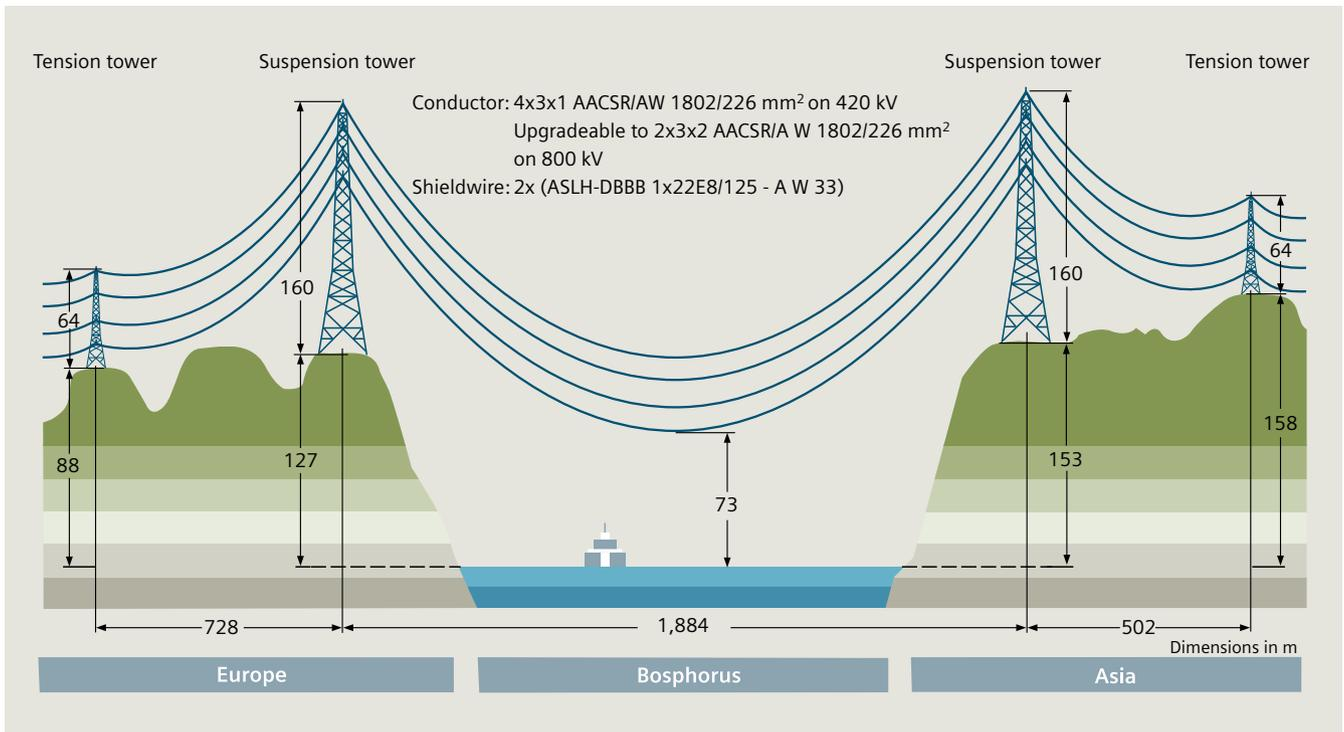
Fig. 2.2-75: 420/800 kV line across the Bosphorus, longitudinal profile
