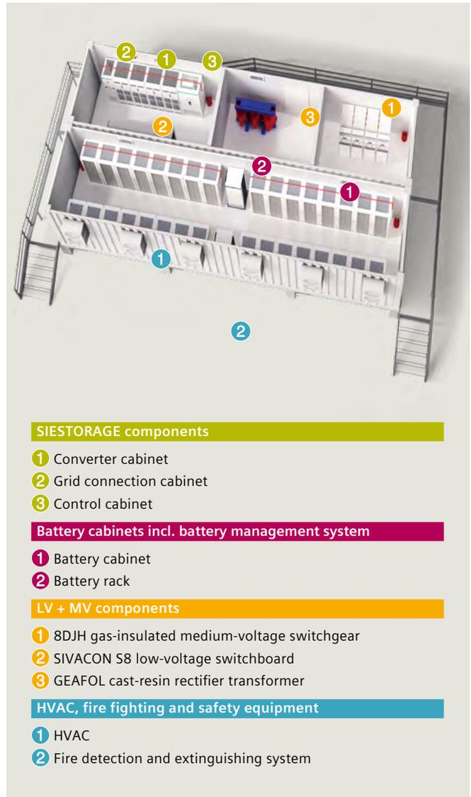
Fig. 2.3-12: Example of a typical containerized comprehensive solution
