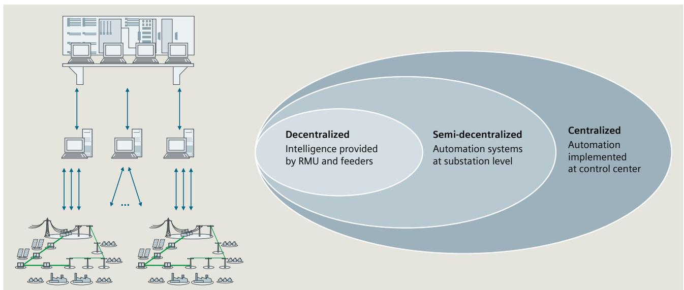
Fig. 6.6-14: Semi-decentralized architecture
