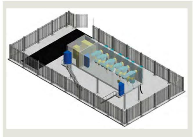
Fig. 2.2-14: 320 kV containerized arrangement
