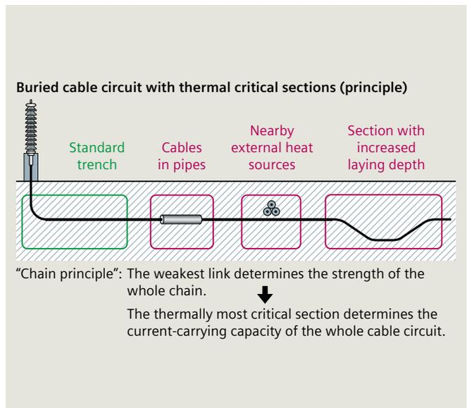
Fig. 2.2-60: Different laying arrangements in ground
