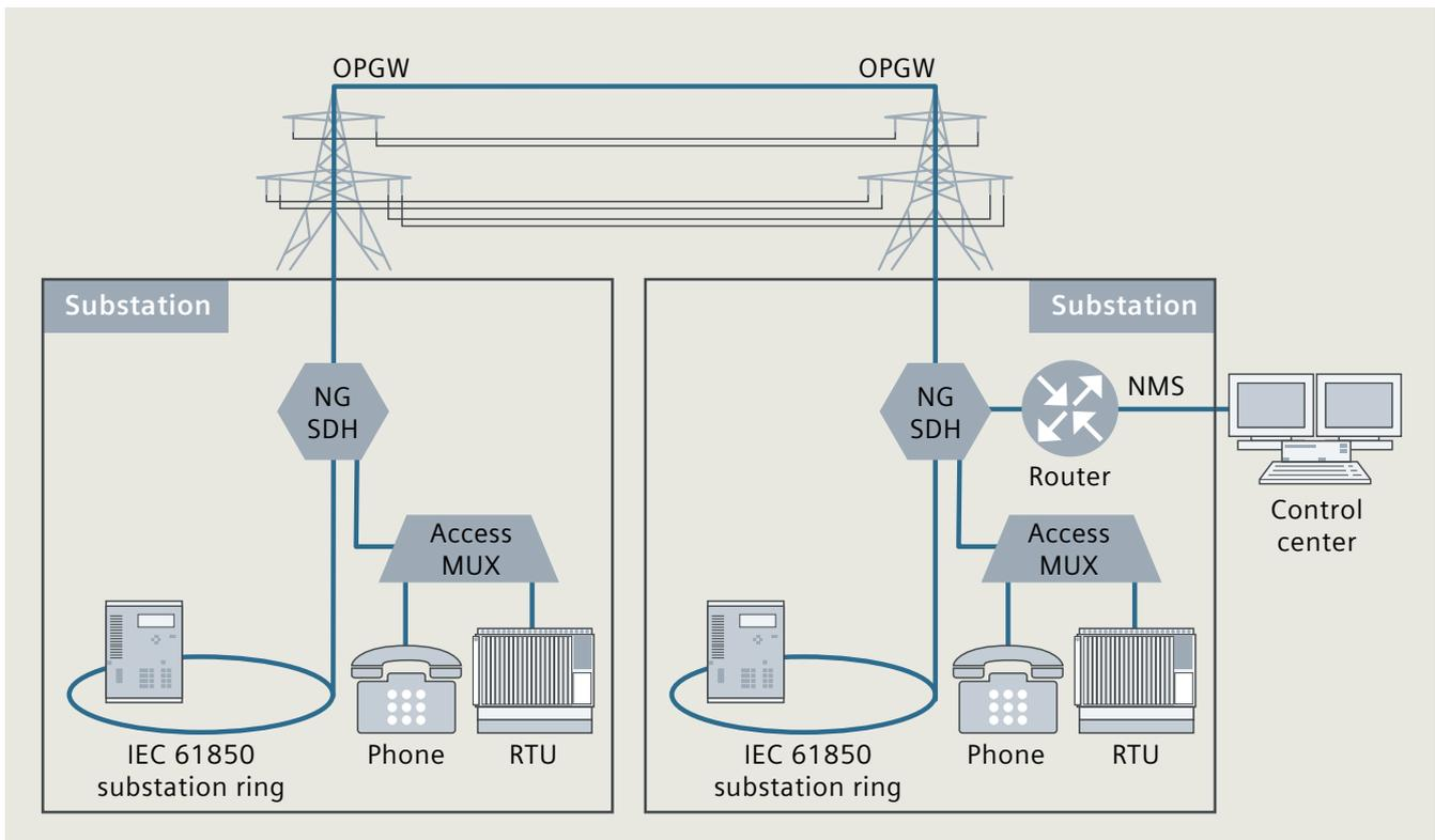
Fig. 8.1-1: Typical NG SDH solution for transmission grids
