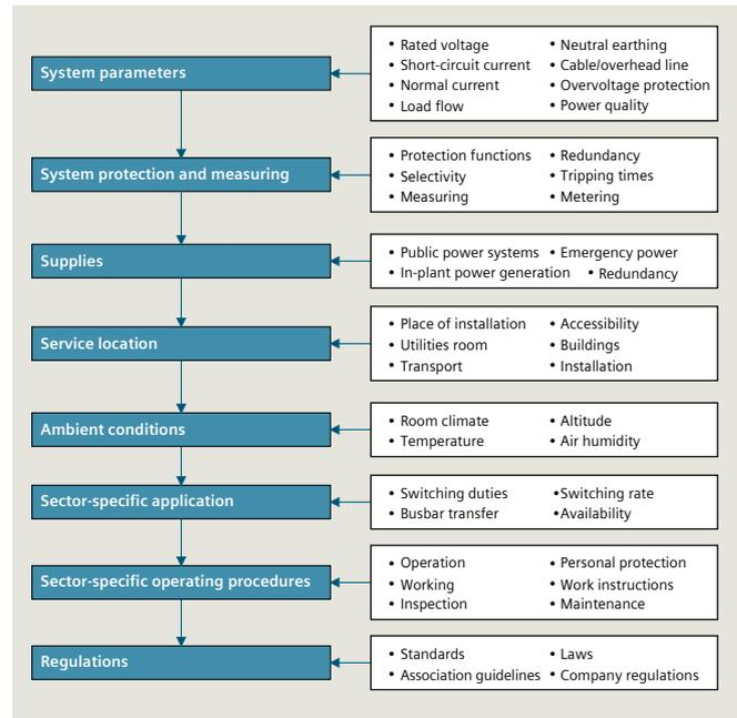
Fig. 3.2-4: Influencing factors and stresses on the switchgear
