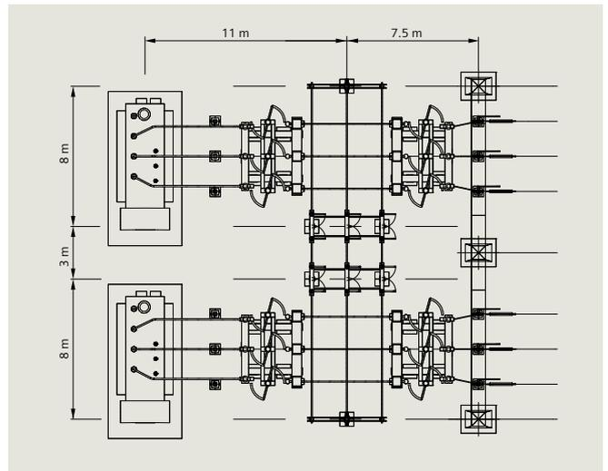
Fig. 3.1-24: SIMOBREAKER (schematic)
