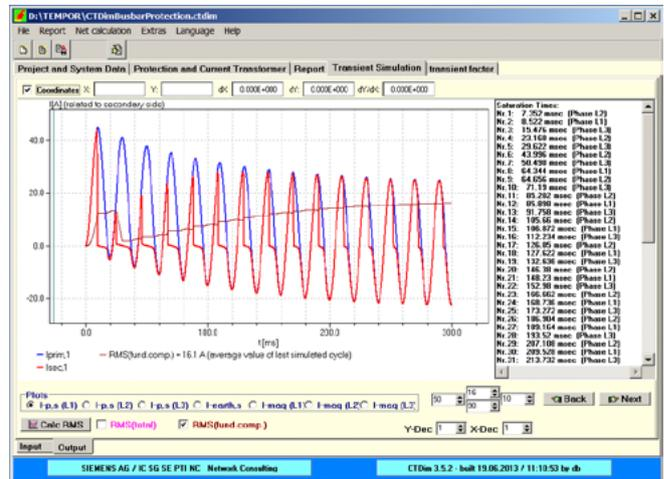
Fig. 9.4-9: CTDim: results of a transient simulation
