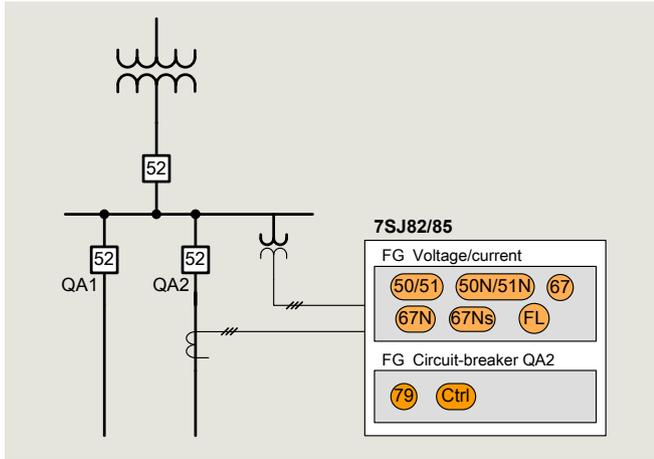
Fig. 6.2-31: Medium-voltage application for all system grounding types
