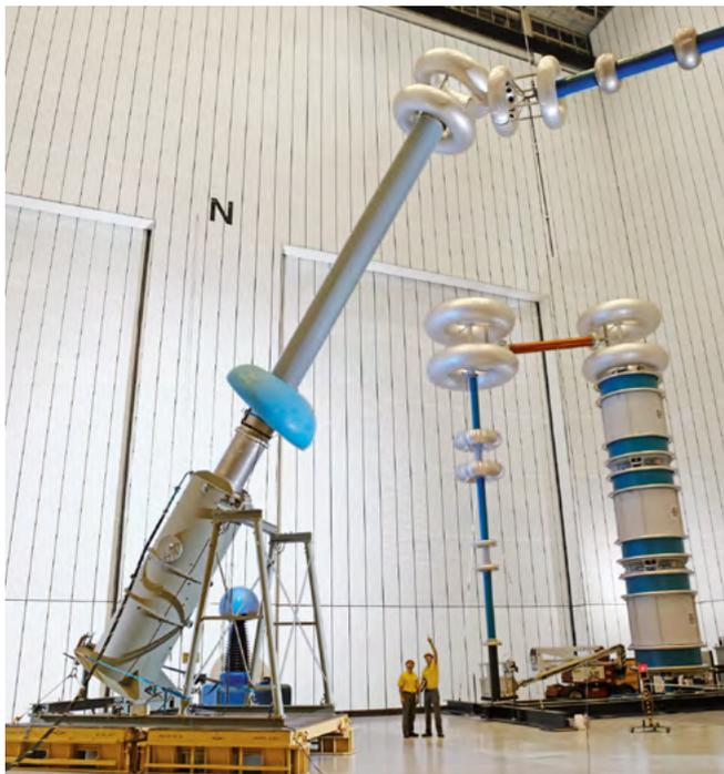
Fig. 4.2-46: Transformer bushing – 800 kV UHVDC – project Yunnan-Guangdong, China
