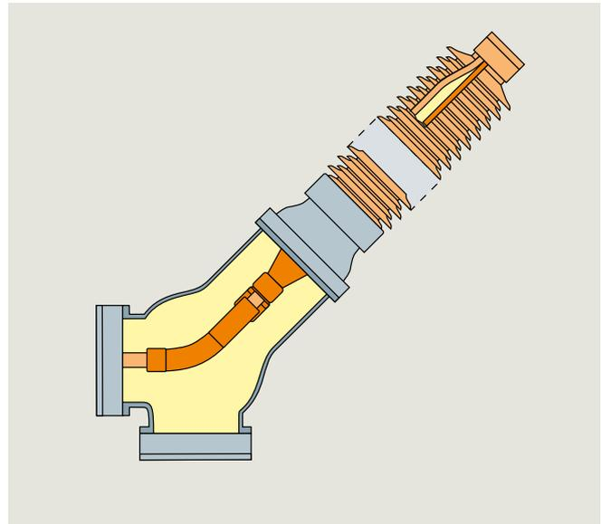
Fig. 3.1-45: Overhead-line terminations: High-voltage bushings are used for the SF<sub>6</sub>-to-air transition. The bushings can be matched to specific requirements with regard to clearance and creepage distances. They are connected to the switchgear by means of angular-type modules of variable design
