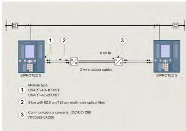
Fig. 6.5-18: Protection communication via a copper connection
