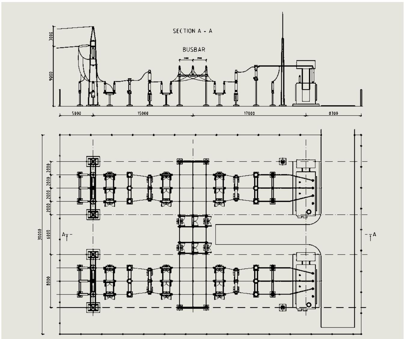
Fig. 3.1-11: H-arrangement 110 kV
