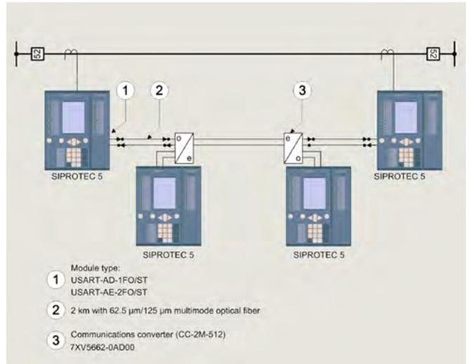
Fig. 6.5-20: Protection communication via single-mode fiber and repeater
