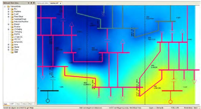
Fig. 9.4-1: Visualizing PSS®E results using single-line diagram contouring
