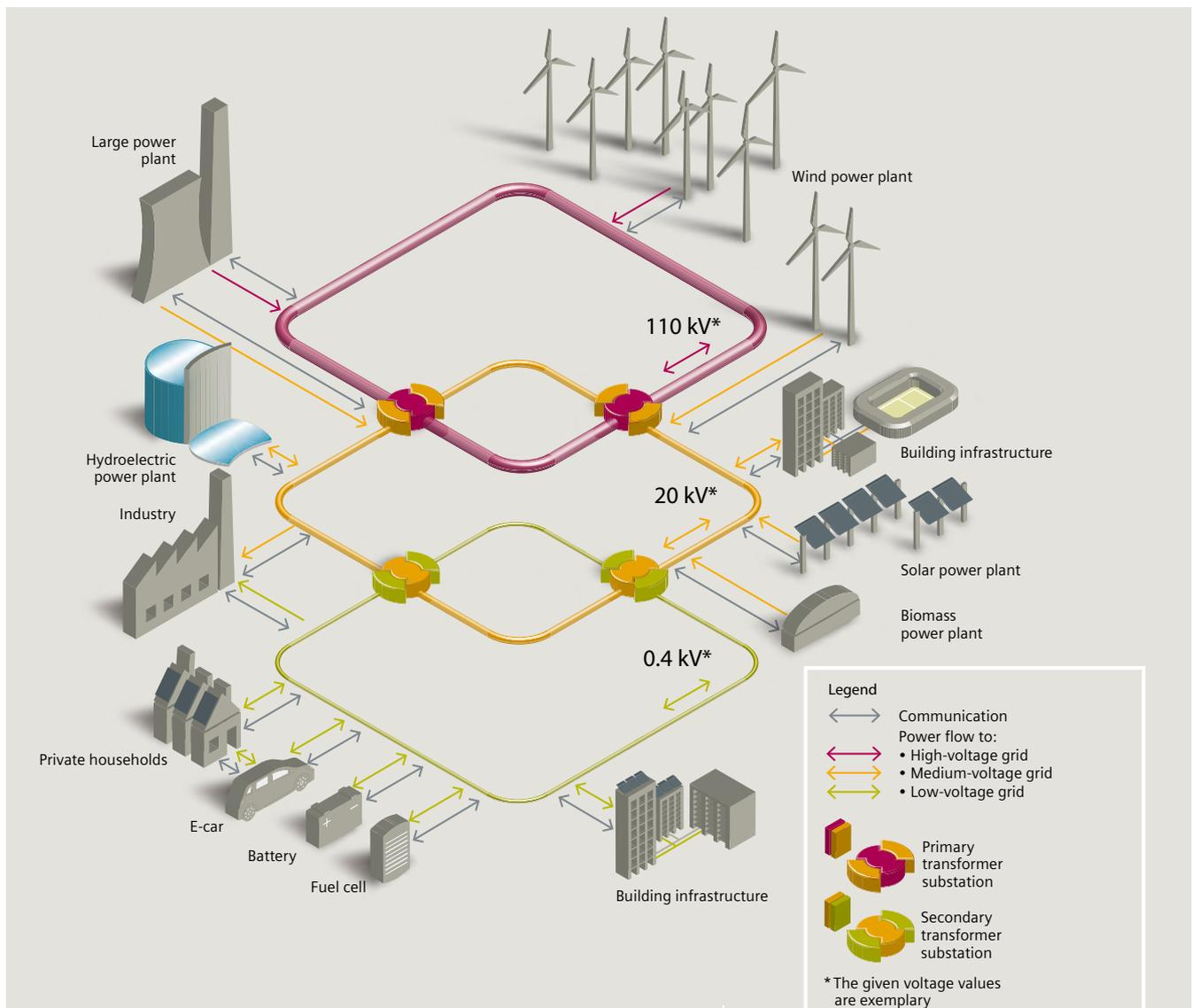
Fig. 2.6-1: Active distribution grid with intelligent transformer substations
