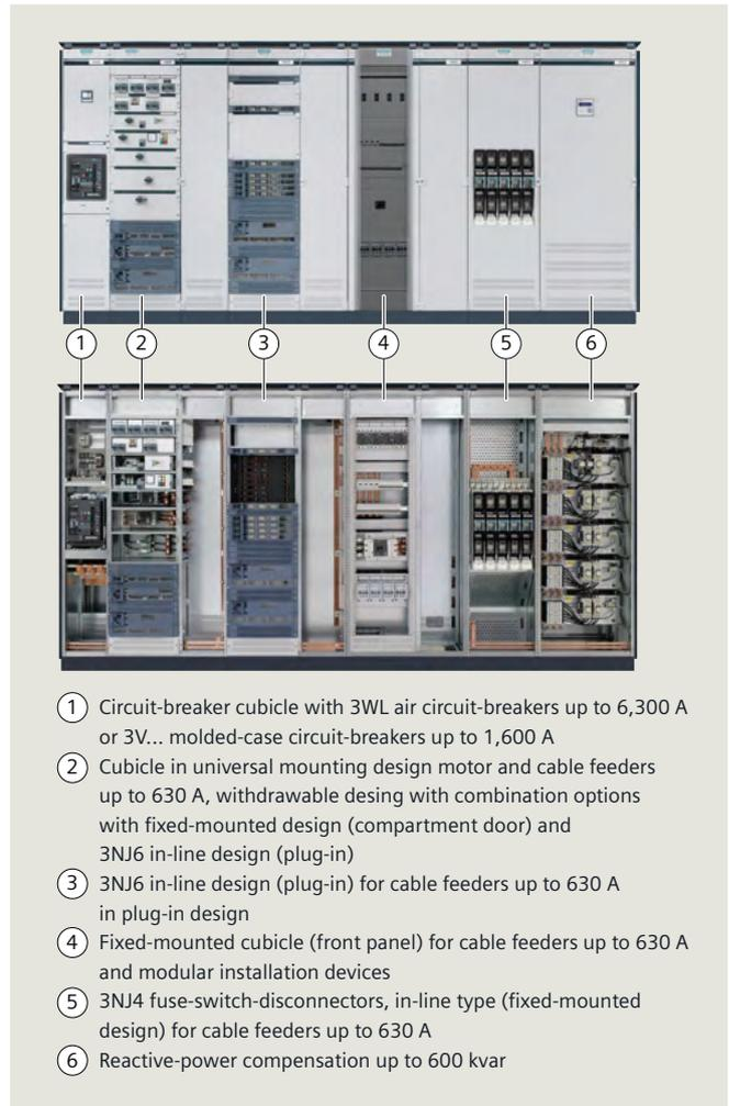
Fig. 3.3-5: The following mounting designs (1-6) are available
