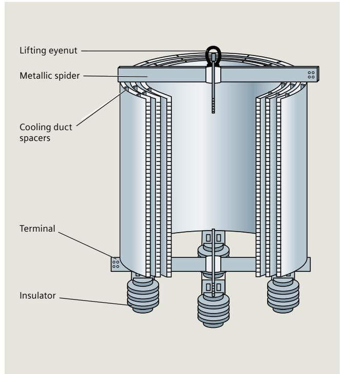
Fig. 4.2-32: Typical Trench air-core dry-type reactor construction
