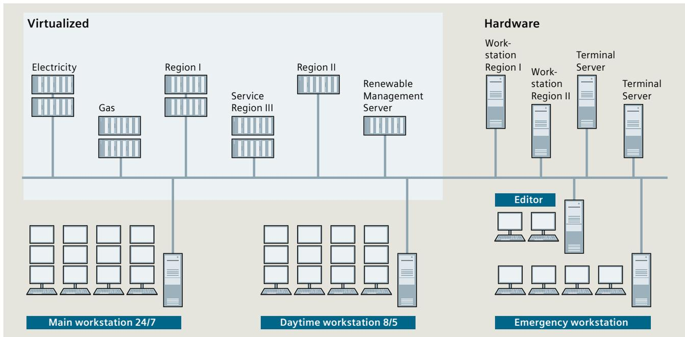
Fig. 6.6-23: Flexibility and scalability of control center solutions
