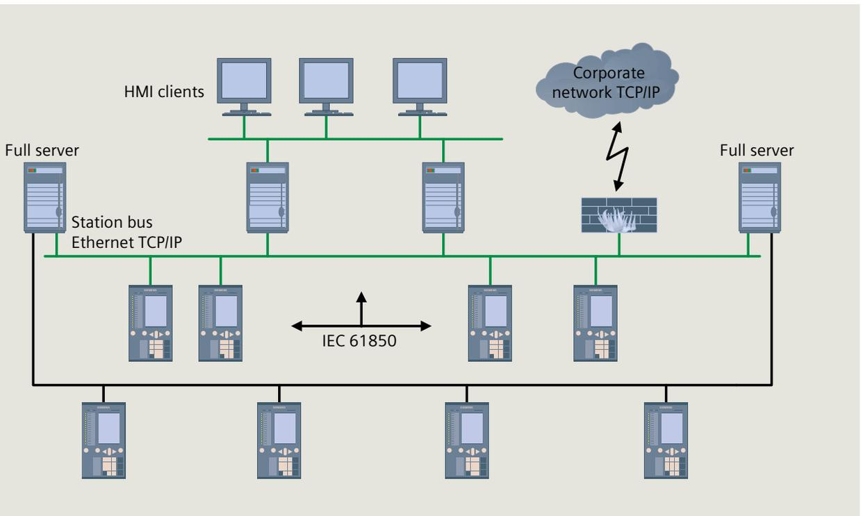
Fig. 6.3-6: Typical redundant configuration: Full server and HMI server are based on a redundant structure to boost availability
