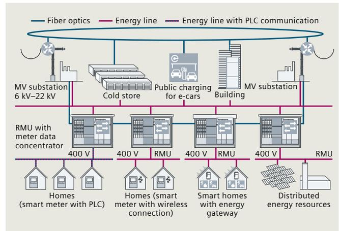
Fig. 8.3-2: Fiber-optic infrastructure for distribution network
