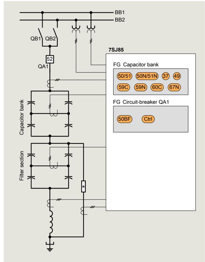
Fig. 6.2-54: Protection of an MSCDN capacitor bank
