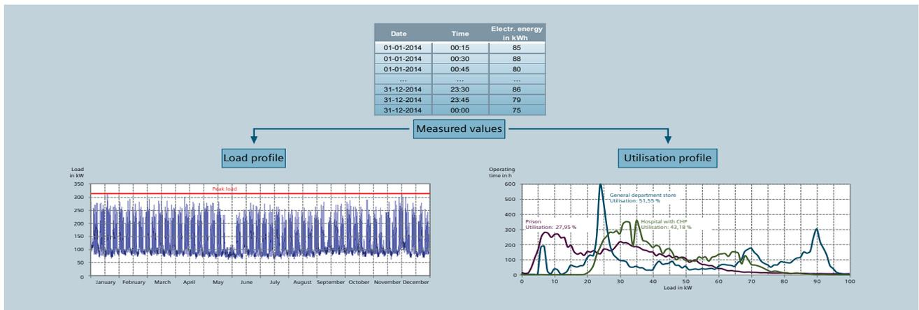
The utilisation profile directly supplies the data for determining transformer loss and the corresponding loss energy (power and corresponding hours).
