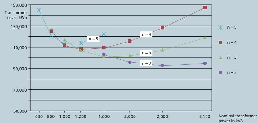
The lowest energy losses are always seen in a configuration with  $n = 2$ . It is evident that the larger transformers tend to become more efficient under an increasing mean load, however at an overall higher level of energy loss. For example, for the office building, the configuration featuring two forced-ventilated 1,600-kVA transformers is energetically the most favourable one, whereas for the metal-processing factory, the two 2,500-kVA transformers show the lowest energy losses.
