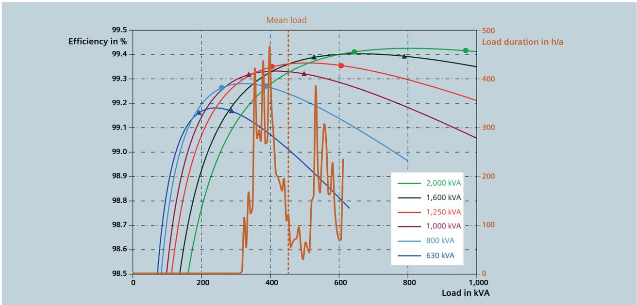
For more precise interpretations, the transformer losses integrated over the corresponding utilisation profile are compared with those related to different transformer ratings as in Fig. 6. You can see that – as opposed to the simple comparison of efficiency curves with mean load situations in Fig. 4 and Fig. 5 – the transformers featuring a somewhat higher rating would have the lowest energy losses.
