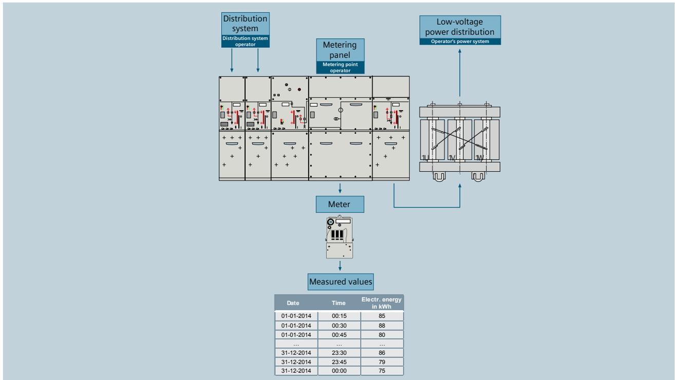
Fig. 3: Creation of load and utilisation profiles from the measurement data
