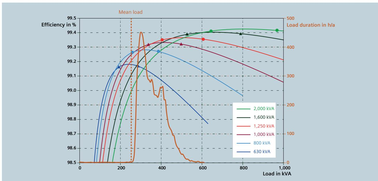
Fig. 5: Utilisation profile of a commercial enterprise and comparison of efficiency curves of several transformers in compliance with IEC 60076-20 (VDE 0532-76-20)
