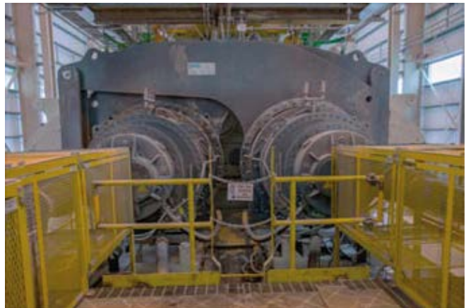
Figure 1: Typical mechanical Drive Train of a large HPGR, powered up by two squirrel cage induction motors with variable frequency converters
