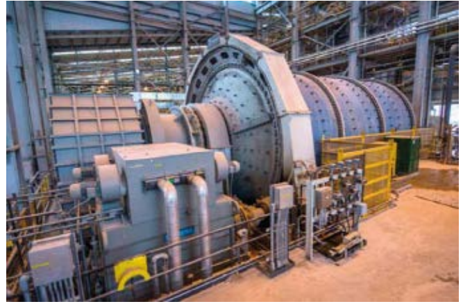
Figure 3: Dual pinion ball mill with 6500 kW Low Speed Squirrel Cage Induction motors using VFC
