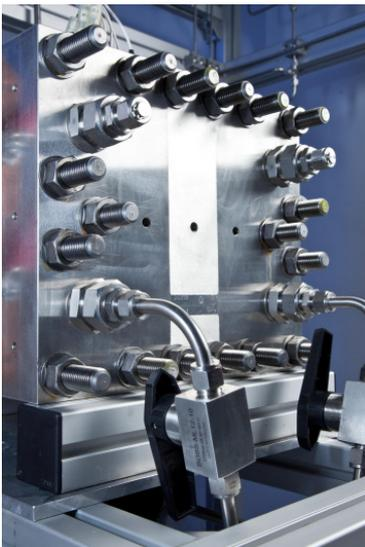
Hydrogen electrolyzer: Detailed view of the PEM stack with its cells and membranes.
