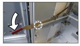
Fig. 251: Pushing the handle downwards to end position
