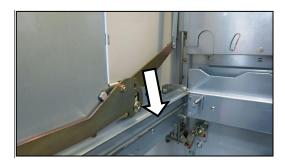
Fig. 250: Pushing on the slip-on lever
