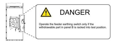
Fig. 163: High-voltage door of panel A:
