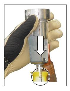
Fig. 334: Plugging the tulip onto the earthing rod
