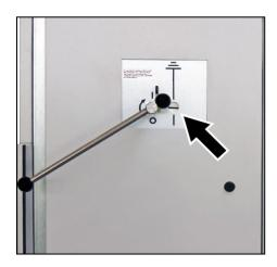
Fig. 246: Operating lever in end position
