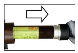
Fig. 207: Pulling out the protection fuse-link
