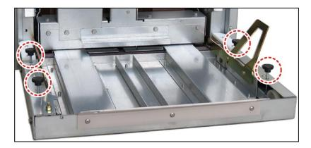
Fig. 186: Adjusting the height with the bolts
