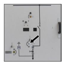
Fig. 48: Actuating opening for racking the withdrawable circuit-breaker
