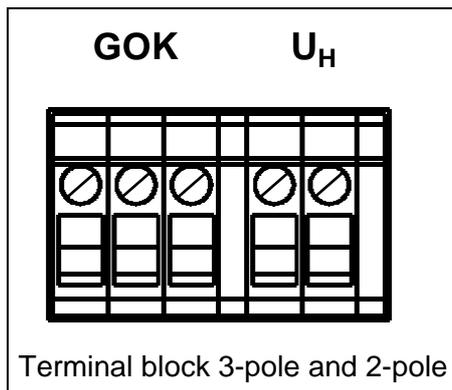
Figure 6 Terminal blocks with screw-type terminals
