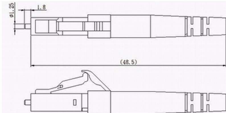
Figure 10 Single LC-connection for the bidirectional FO-Repeater
