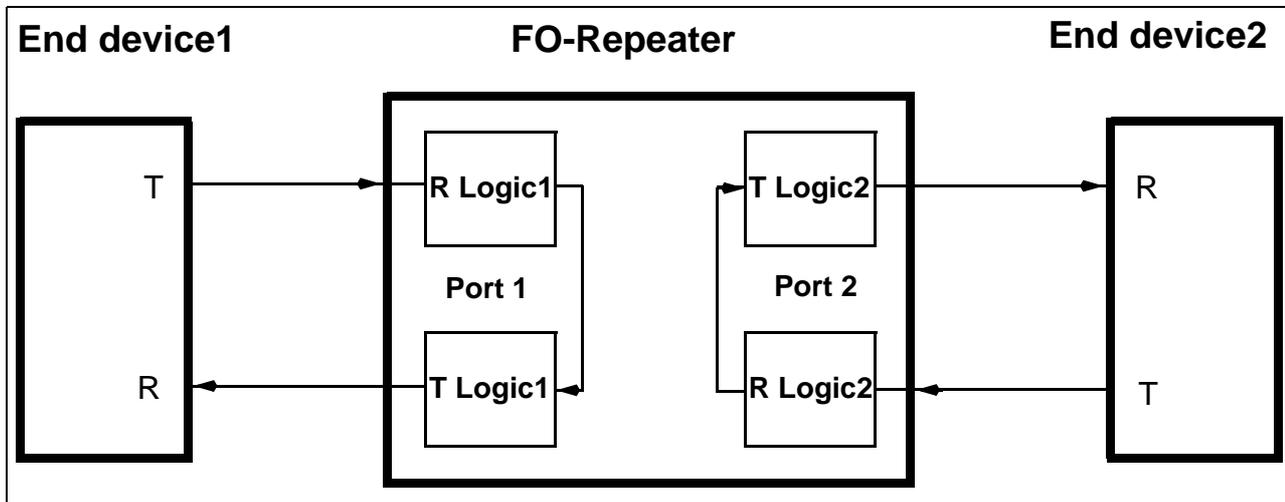
Figure 13 Diagram of the *Echo Mode* operating mode
