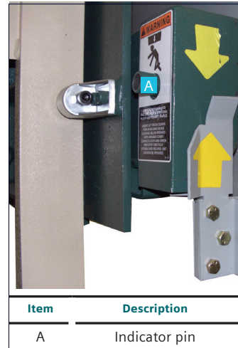
Figure 44: Lift truck engaged - note position of indicator pin
