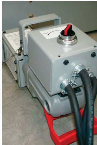
Figure 61: Electrical racking device
