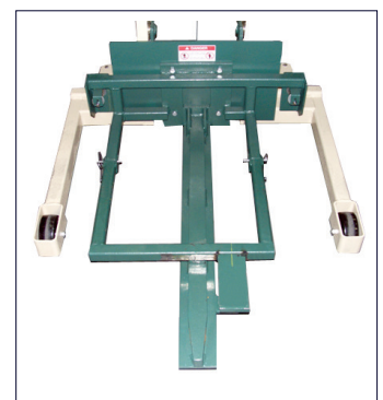
Figure 52: Lift truck forks with auxiliary tray adapter (for up to 50 kA)
