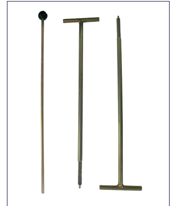
Figure 50: Rollout racking tools and manual trip rod
