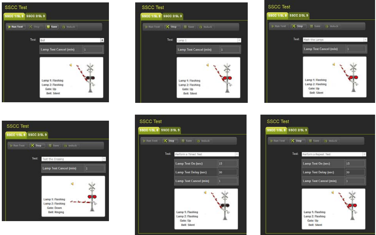
Figure 3-68 CPU III Web UI – Calibration & Adjustment – SSCC – SSCC Test Screens
