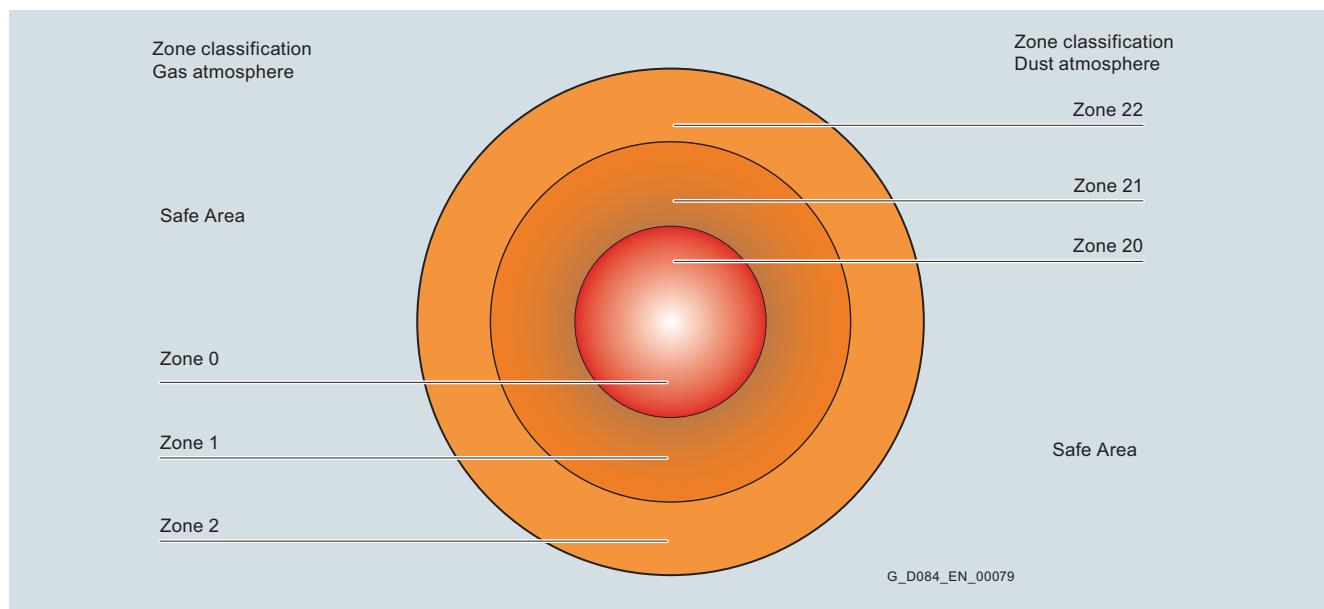
Depending on the particular zone and therefore the associated hazard, operating equipment must comply with defined minimum requirements regarding the type of protection. The different types of protection require corresponding measures to prevent ignition that should be implemented at the generator in order to prevent that a surrounding explosive atmosphere is ignited.
