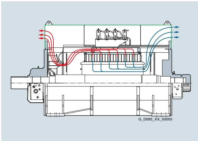
**Air/water heat exchanger (IC81W)**
