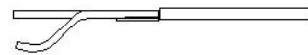
REMOVING TOOL FOR RETAINING CLIP J10648/1 (for relays with pressed steel handles)
