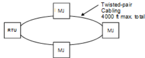
Figure 5-4: RS-485 Loop Topology
