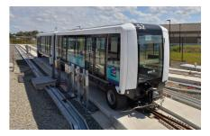
Automated People Mover Rennes The Rennes Line B has very low headways of 67 seconds at peak times, with three car trains, and guarantees high availability of 99.7%. The highly scalable, modular system can be extended to a 3-car configuration. Maximized interior space and latest digital passenger information leads to an enhanced passenger experience.
