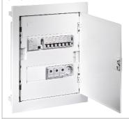
Flush-mounting, degree of protection IP 30, safety class 2, for use up to 63 A These distribution boards are tested in accordance with DIN VDE 0603, DIN 43871, IEC 60439-3 for use in countries using DIN systems.
