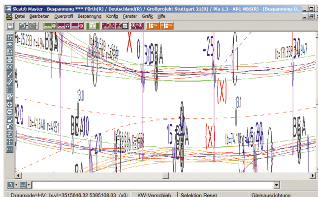
Descalped view with pantograph range and run of wind deflection
