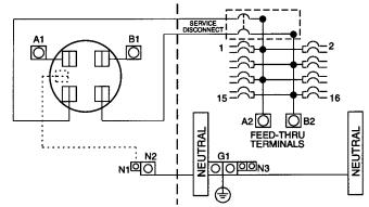
SHORT CIRCUIT CURRENT RATING (WATTHOUR METER NOT INCLUDED IN SHORT CIRCUIT RATING) SHOULD CHARLENT HATING (WAT HOUR METER NOT INCLUDED IN SHOULD INCLUDENT HATING)
