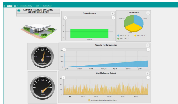
Electrical meter dashboards visualize real-time data about demand, consumption and current output.
