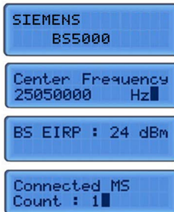
Figure 6-1 Base Station LCD Screen – Remote Station Connection
