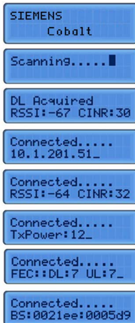
Figure 6-8 Remote Station Connection Process LCD Screens
