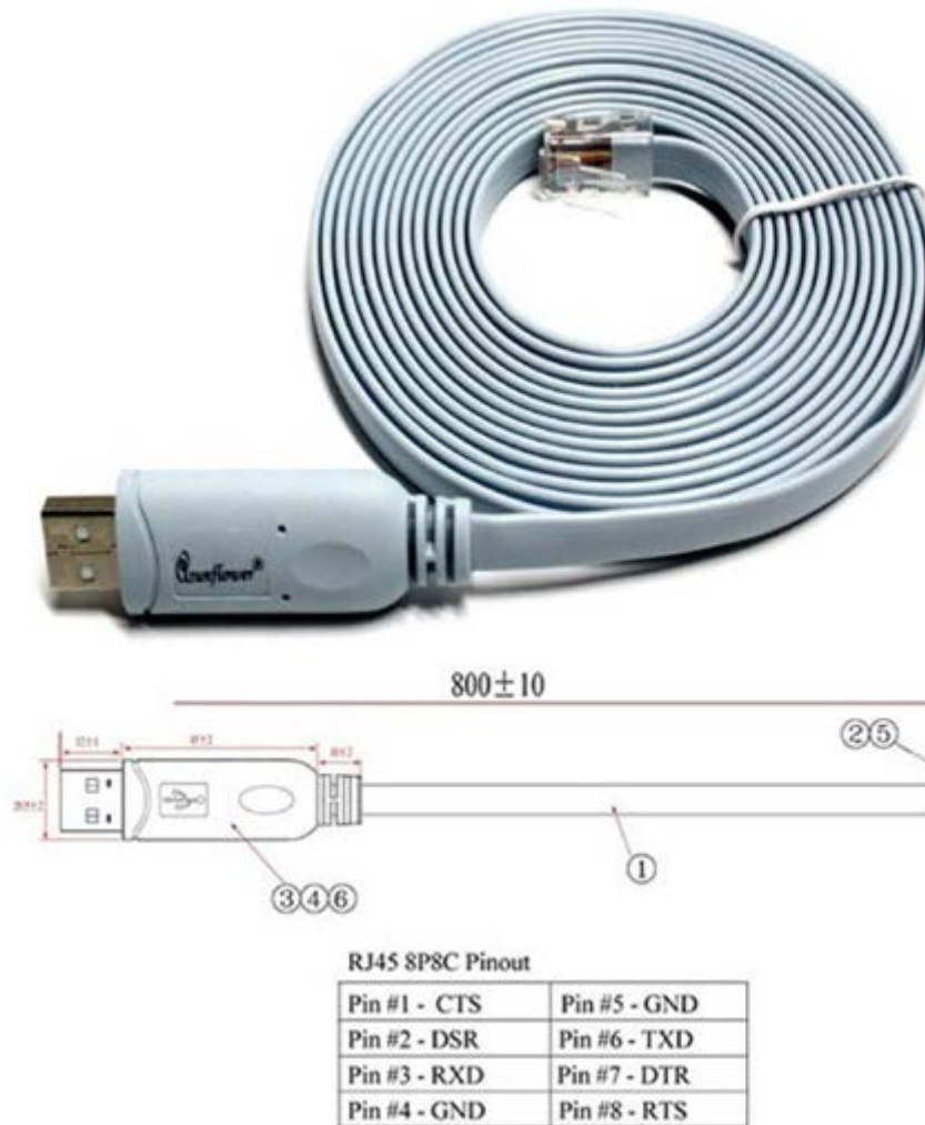
Figure 5-1 Console Port Cable (USB to RJ-45)
