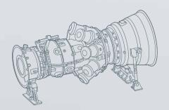
Striking features of the new SGT-750 include its efficiency and ecofriendliness, combined with high availability and reliability. The turbine has an electrical efficiency of 39.5% and achieves an efficiency of 40.7% when used as a mechanical drive. When exhaust heat is used in a combined heat and power system, fuel efficiency can be as high as 95%.
