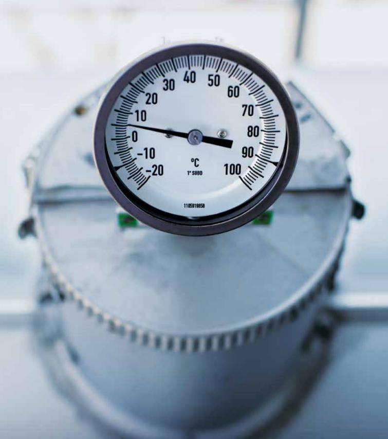
**Combating ice with 459°C** | The Joule-Thomson effect describes the phenomenon whereby natural gas in pipelines cools when the pressure is reduced. At temperatures near the freezing point, a great deal of energy is needed to heat the gas in order to prevent icing. In the past, gas-fired boiler plants with a heat output of 40 megawatts each were used for this purpose. The SGT-750 offers technology that is both
