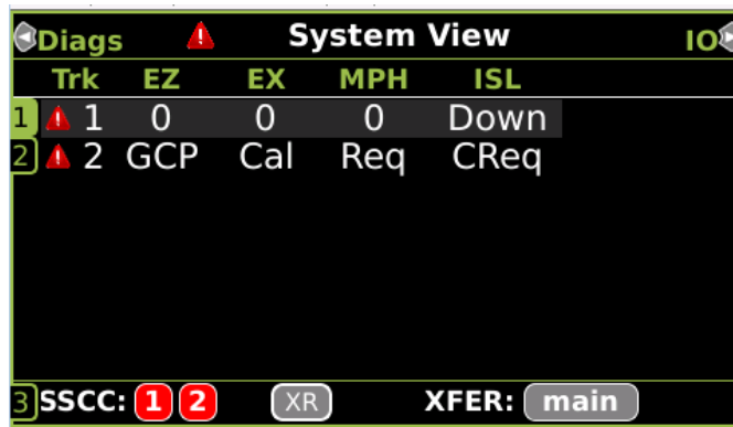
Figure 8 System Screen for GCP 4000 Transfer unhealthy
