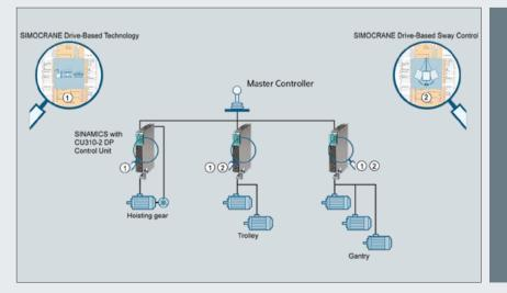
For hoist applications, an encoder is requested for safety reasons and for providing pendulum length to cross travel (trolley) and long travel (gantry).
