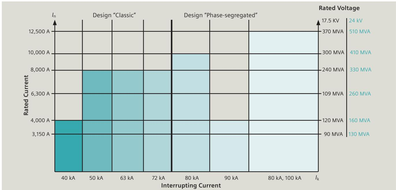
Replacement vacuum circuit breakers for generator switching applications for 17 kV and 24 kV. Graph represents ratings and offerings covering Siemens' complete line of GCBs.
