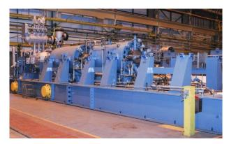
Above: Multiple DATUM compressors, like those shown in this photo, will compress synthesis gas to high pressures.
