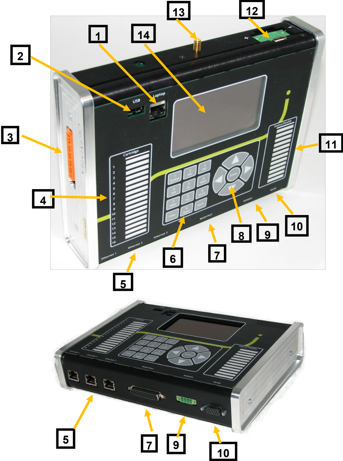
Figure 1-2 Console Indicator and Control Locations
