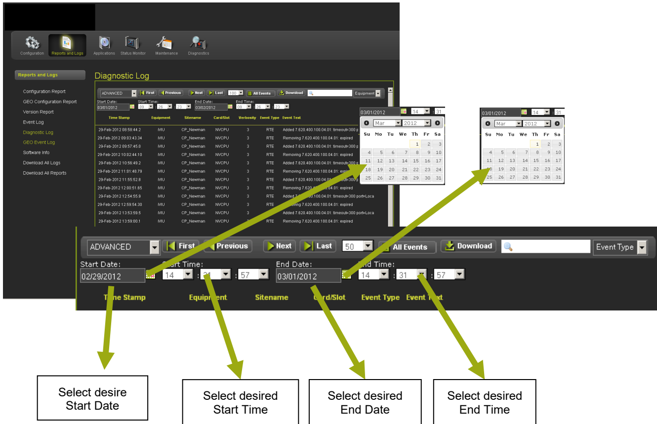
Figure 4-52 Diagnostic Log - Advanced
