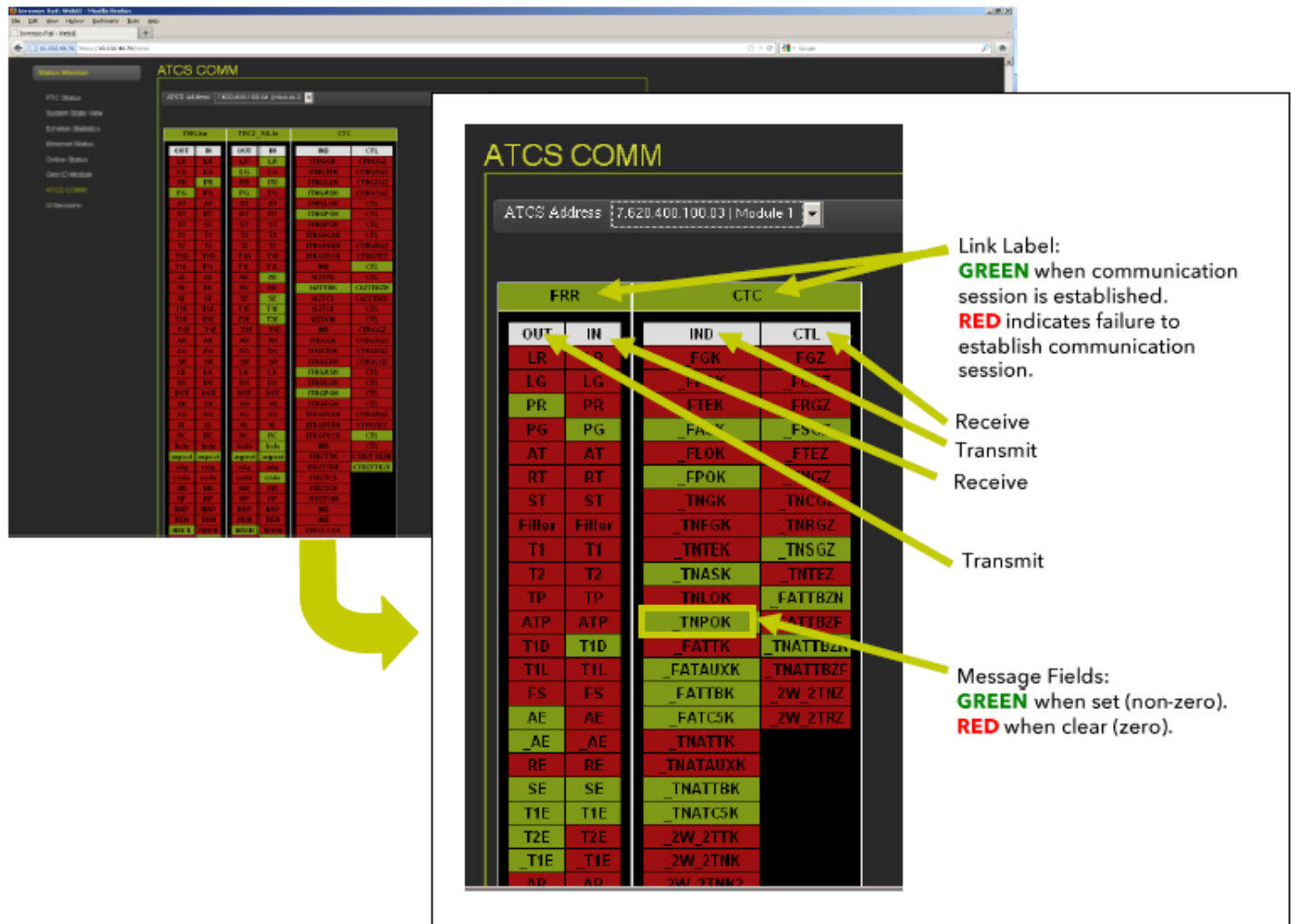
Figure 4-102 ATCS Communications Links
