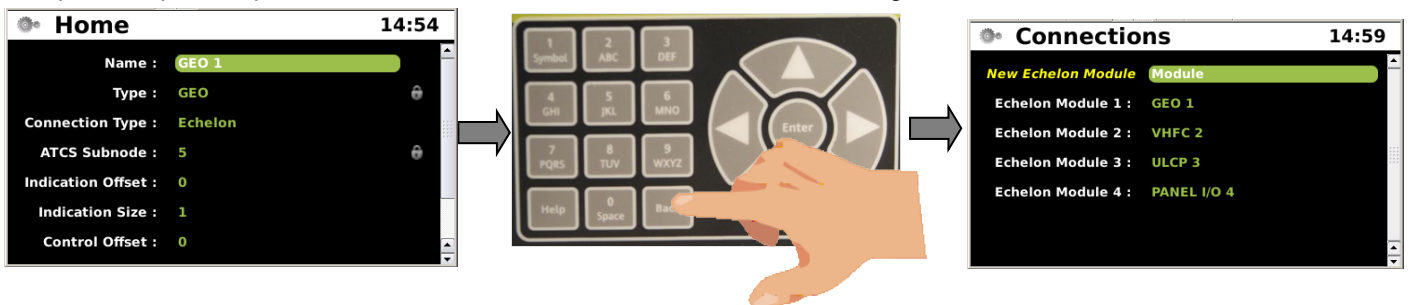
Figure 5-28 Module Menu - Connections - Module Configure Complete
