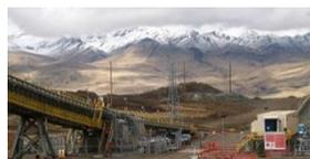
Siemens is undertaking the engineering, design, production and supply of the electrical equipment for the Oyu Tolgoi copper mine conveyor system. The new system extends the existing opencast mining facility and is expected to bring 95,000 tons of copper ore to the surface per day. The conveyor system has to overcome a difference in height of almost 1,400 m. The order value is in the tens of millions of Euros.
