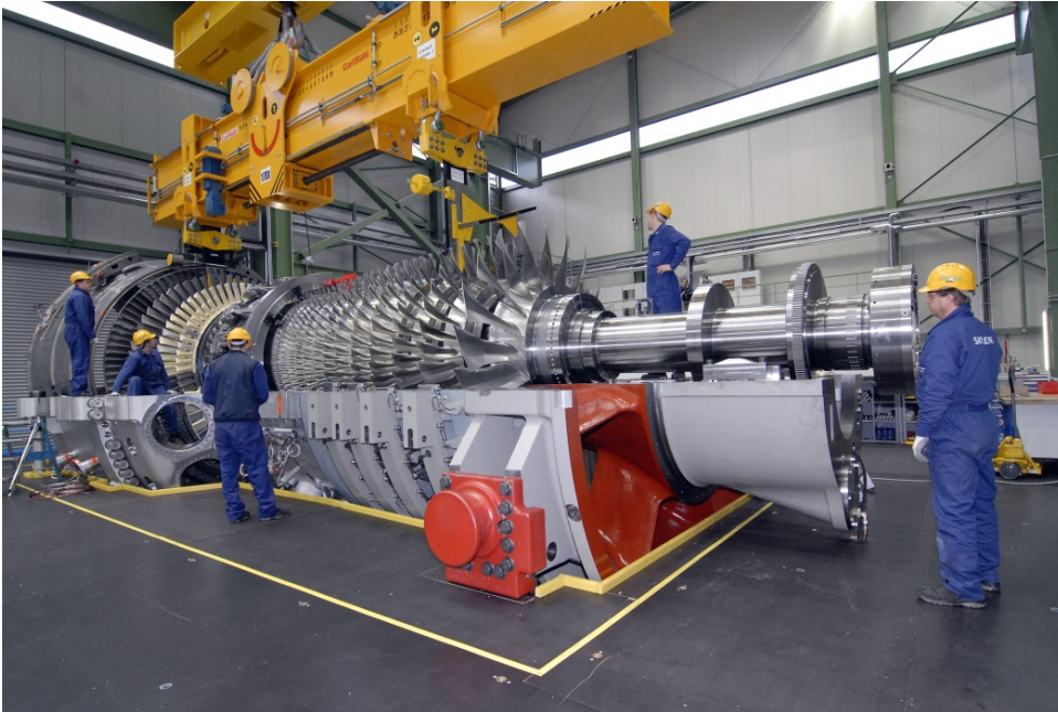
Final Assembly of SGT5-8000H in the Siemens gas turbine factory in Berlin
