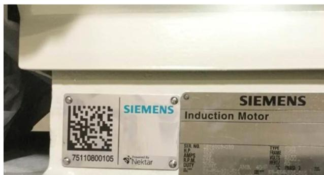
Figure 1. QR codes are used with geo-location to track an asset’s physical location, as well as maintenance and service history.
