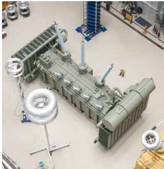
Transformer in the extra-high voltage test hall
