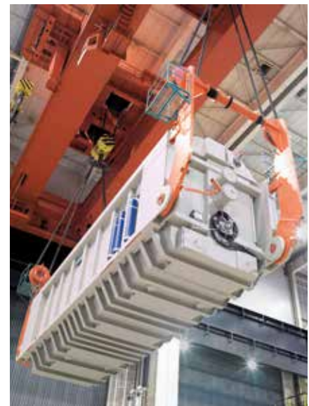
This tank is specially built for transport on a Schnabel car
