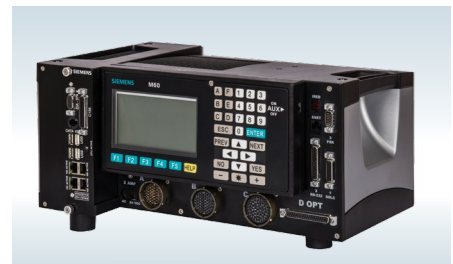
Siemens M60 ATC controller running SEPAC local controller software
