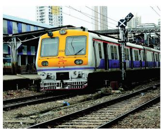
Regenerative breaking helps save energy by converting mechanical energy into electrical energy, which goes to the power supply grid.
