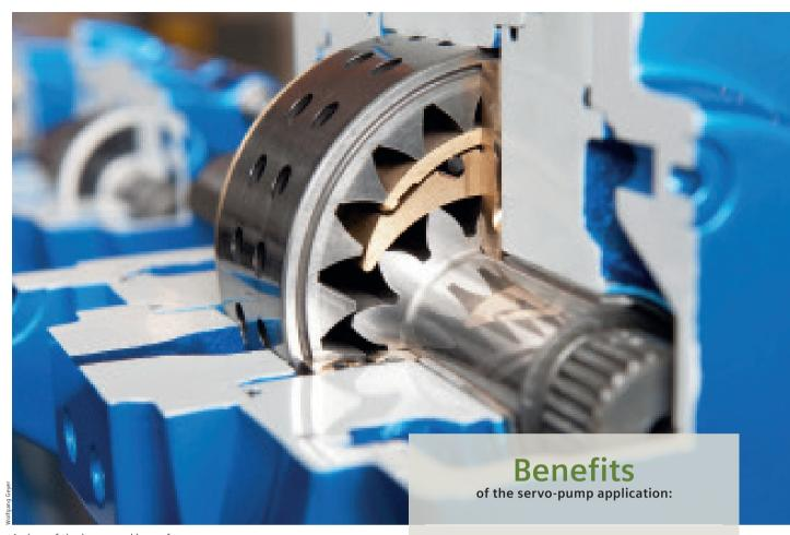
A view of the inner workings of a gear pump whose operation is controlled by a servomotor
