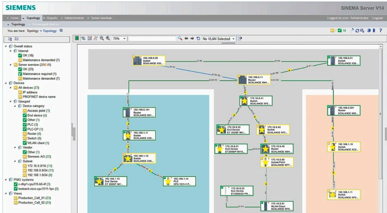
During operation, the automatically generated plant topology SINEMA serves as reference during every cyclical query, on the basis of which the system recognizes and displays every change.
