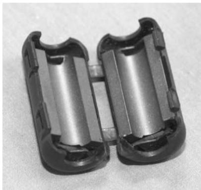
**Figure 1. Clamp-on EMI Filter (open)**
