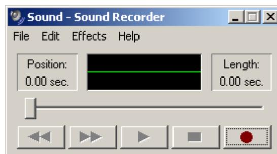
Individual words and phrases recorded with the Sound Recorder utility must be saved in the **CCITT u-Law** format, with **8 kHz, 8-bit, Mono** attributes.
