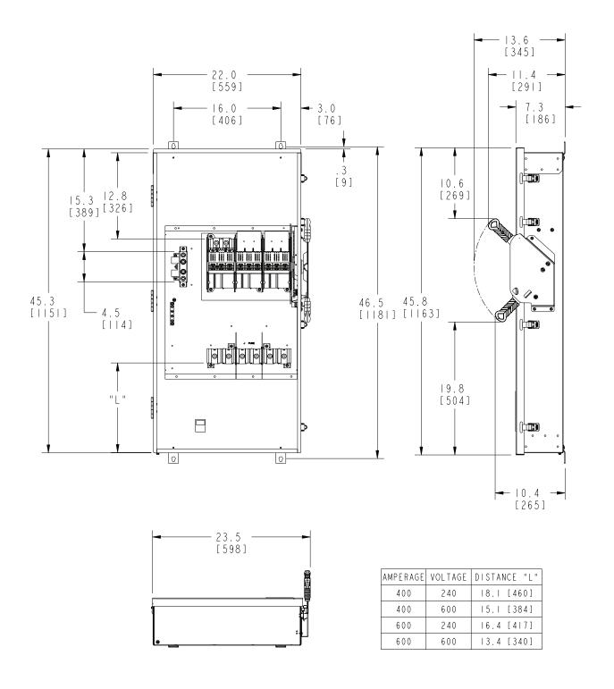
Dimensions shown in inches and millimeters [ ]. Dimensions shown accurate to  $\pm$  1/8 inch.
