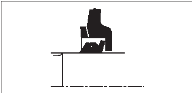
Dismantling the V-ring and adjacent protecting ring
