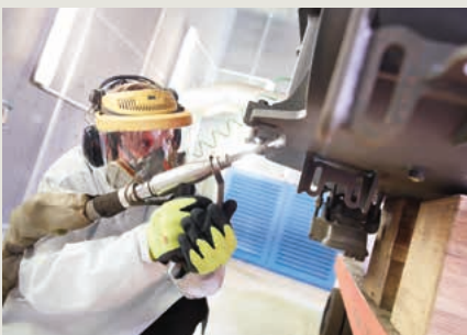
Cleaning cabin Cleaning up the bogies and their components with dry ice.
