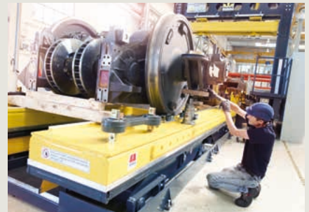
Pressure rig Here we ensure an even load distribution of wheel disc on track.
