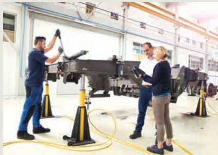
Disassembly and assembly stands Our extendable hydraulic cylinders can be used flexibly.
