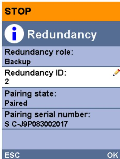
Figure 9-3 Assigning redundancy IDs
