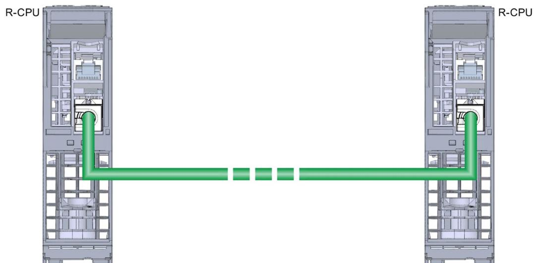
Figure 5-6 PROFINET interface X1 P2 R: Connecting R-CPU (bottom view)
