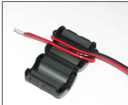
Figure 3-6 EMI Filter Installation (showing wire loops)
