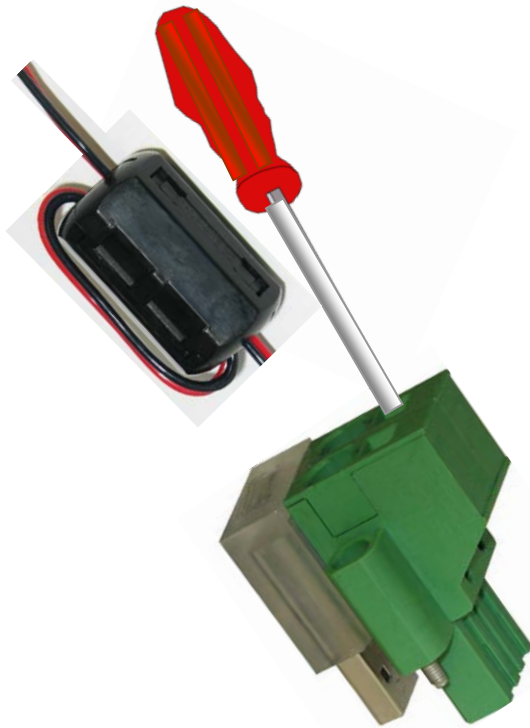
Figure 3-4 Power Conductor Wire Installation
