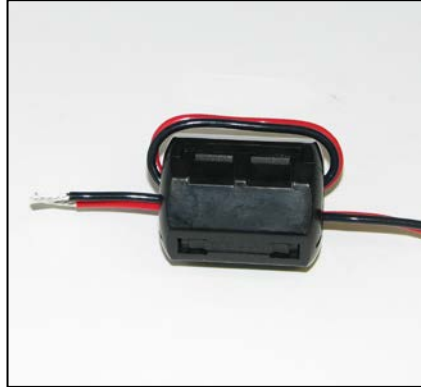
Figure 3-7 EMI Filter Installed
