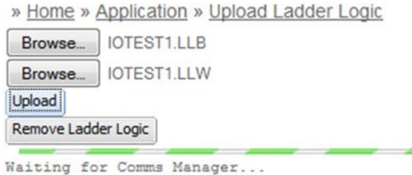
Figure 4-104 Upload Ladder Logic Files – Uploading in Progress
