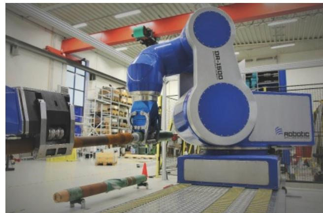
Multi-axis drill floor robot designed for handling pipes and drill heads
