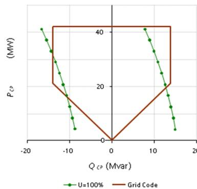
Figure 1: Example of reactive power capability curves
