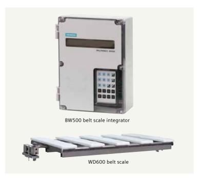
As material is moving along the conveyor belt and travels over the belt scale, it exerts a force proportional to the material load through the suspended weighbridge to the load cells.
