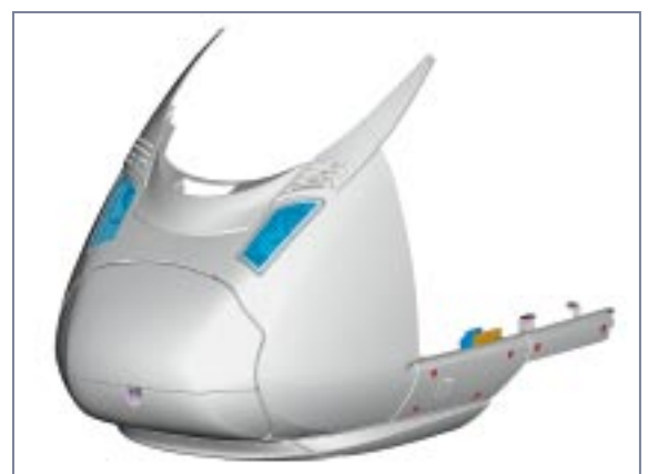
Fig. 6: Newly designed nose shell with coupler doors and headlights
