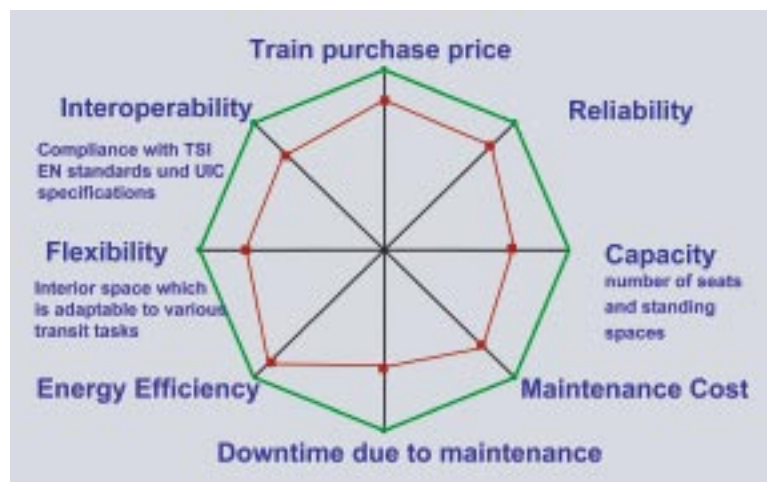
Fig. 3: Target dimensions for the development of the Velaro platform
