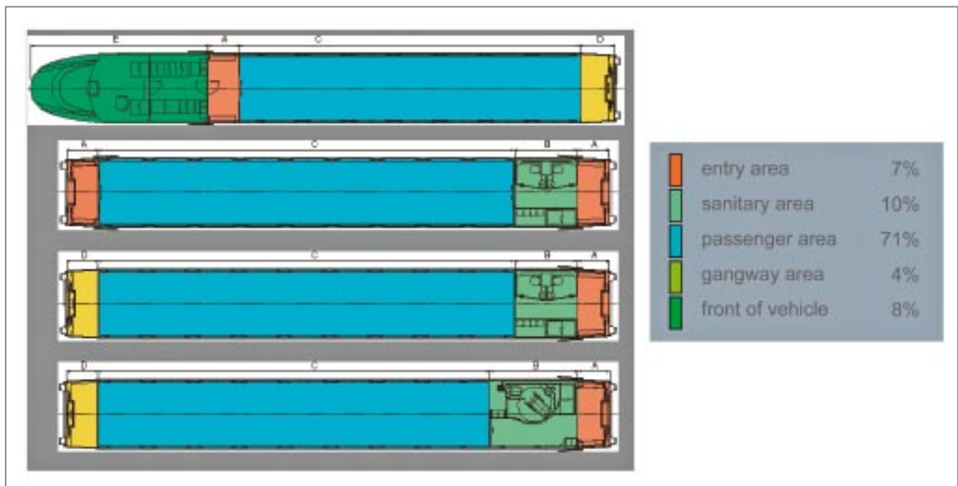
Fig. 16: "Empty tube" principle for the largest possible usable floor area
