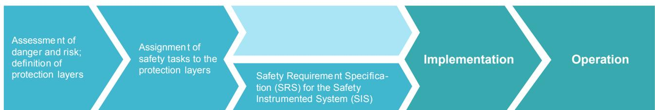
The safety concept for the plant is subsequently produced. During this, the safety tasks are assigned to the various protection layers of the plant.
