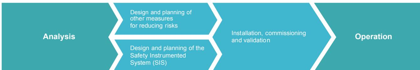
The specified safety functions are implemented during the planning phase. When using the SIMATIC S7 Safety Matrix, the safety functions defined during the analysis phase are presented in the form of a Cause & Effect matrix, which can be used directly to generate the logic required within the SIS.
