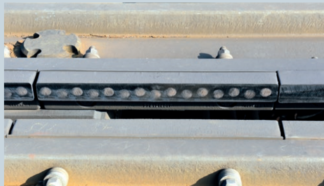
Retarder segment (braking beam with PUCK inserts)
