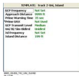
Figure 10-9: TEMPLATE: track “N”-Uni, Island Window with Preemption set to Off and Prime UAX set to Off
