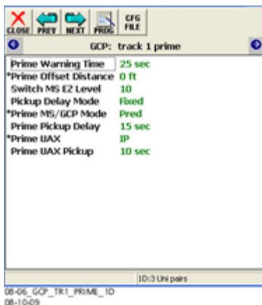
Figure 5-11: GCP: Track 1 prime Screen Prime Warning Time
