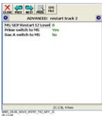
Figure 5-37: Prime Switch to MS on Track 2
