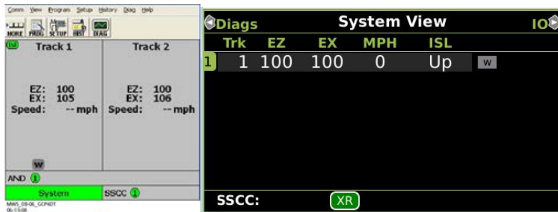
Figure 6-65: 4000 GCP DT Window View and Display View
