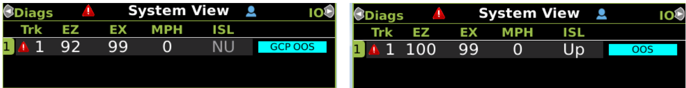
Figure 5-85: OOS Track Status Indications on Display
