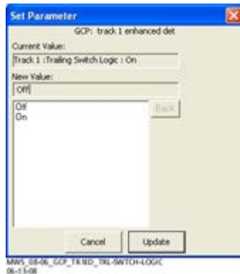
Figure 5-70: Set Trailing Switch Logic Parameter Window
