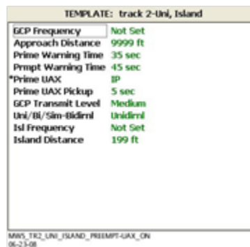
Figure 10-10: TEMPLATE: track “N”–Uni, Island Window with Preemption set to “Advnce” and Prime UAX On
