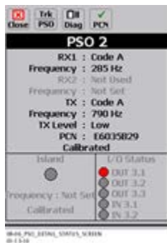
Figure 6-184: PSO Detail Status View Window
