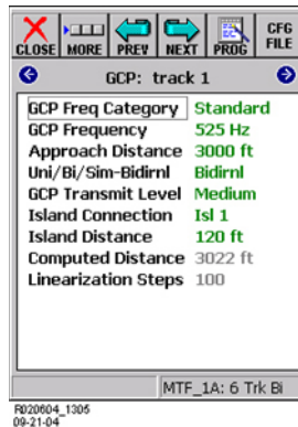
Figure 5-24: GCP: Track 1 Window
