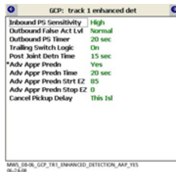
Figure 10-44: GCP: track “N” enhanced det “Adv Appr Predn Yes” Window
