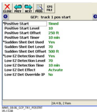
Figure 5-34: Positive Start Programming Window
