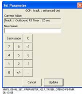
Figure 5-69: Set Outbound PS Timer Parameter Window
