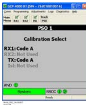
Figure 6-185: PSO Calibration Select Window
