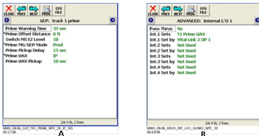
Figure 6-153: (A) UAX Setup for Crossing 2, (B) Internal Connections for Crossing 2
