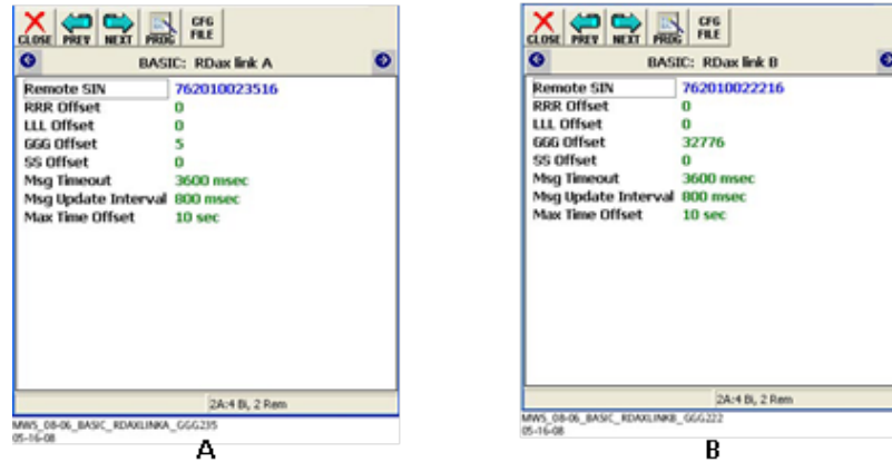
Figure 6-110: Entering DAX Link Offset Values for A: RDAXA; and B: RDAXB
