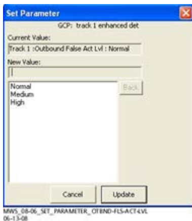
Figure 5-68: Set Outbound False Act Lvl Parameter Window
