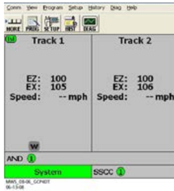
Figure 6-75: GCP 4000 DT Window with Track 1 Wrap On
