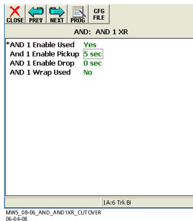
Figure 5-97: AND 1 XR Configuration During Cutover (Train Detection)
