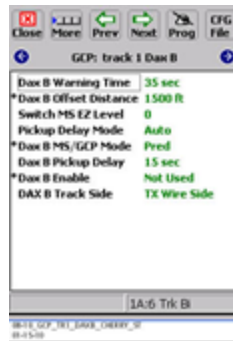
Figure 6-215: Cherry Street (West Approach) Programming: GCP: Track 1 DAX B Window
