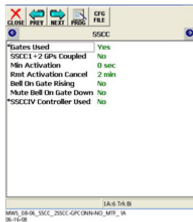
Figure C-15: SSCC Parameter Settings for GP Inputs to Independent Crossing Controllers
