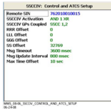
Figure 10-78: SSCCIV: Control and ATCS Setup Window
