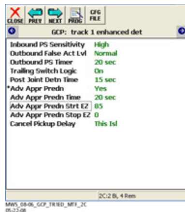
Figure 6-38: The GCP: Track 1 enhanced det "Adv Appr Predn" Window
