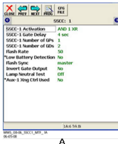
Figure C-20: SSCC Crossing Controller Configuration
