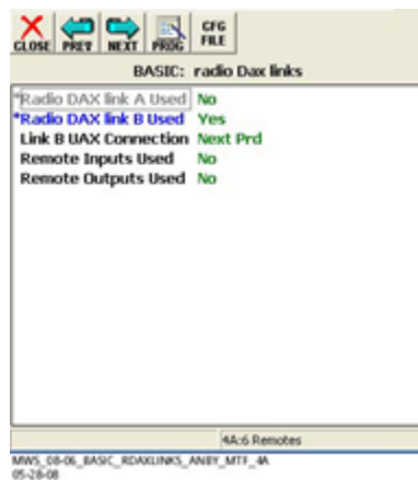
Figure 6-113: Remote 1 (GCP-7) Radio DAX Link Configuration
