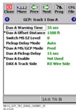
Figure 6-213: Cherry Street (East Approach) Programming: GCP: Track 1 DAX A Window
