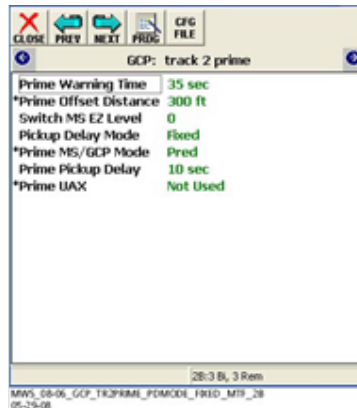
Figure 5-56: T2 Prime is Fixed 10 Second Pickup Delay
