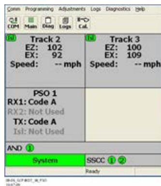
Figure 6-183: Model 4000 GCP DT Window with PSO Summary Data
