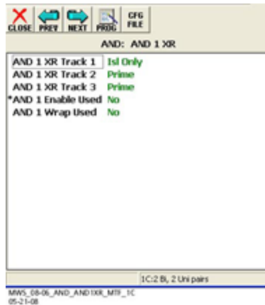
Figure 6-14: AND 1 XR Track 1 Field Set To Island Only
