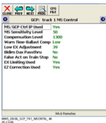
Figure 5-62: MS Sensitivity Level Parameter Adjustment Window
