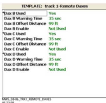
Figure 10-17: TEMPLATE: track “N”- Remote DAXes Window
