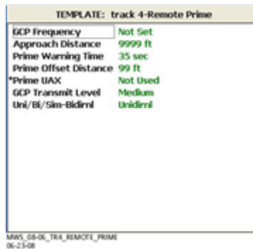
Figure 10-14: TEMPLATE: track “N”-Remote Prime Window with Preemption and Prime UAX set to Off
