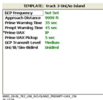
Figure 10-12: TEMPLATE: Track “N”-Uni, No Island Window with Preemption set to “Advnce” and Prime UAX set to On
