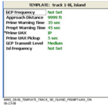
Figure 10-8: TEMPLATE: track “N”-Bi, Island Window with Preemption set to “Advnce” and Prime UAX set to On
