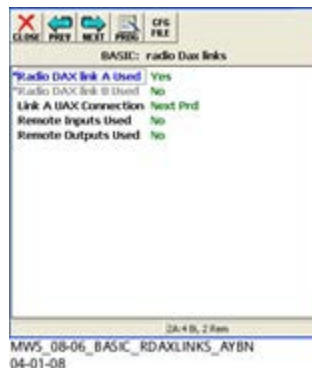
Figure 6-116: Crossing 5 (GCP-5) Radio DAX Link Configuration
