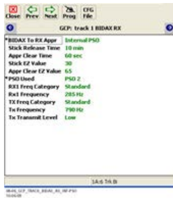
Figure 10-45: GCP: Track “n” BIDAX RX Window
