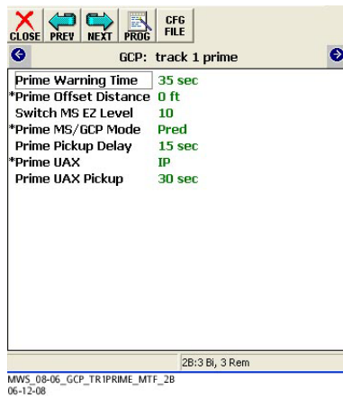
Figure 5-58: Prime Programming Assignment
