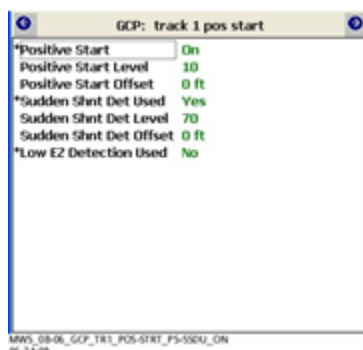
Figure 10-51: GCP: Track “N” pos start “Positive Start and Sudden Shunt Det On” Window
