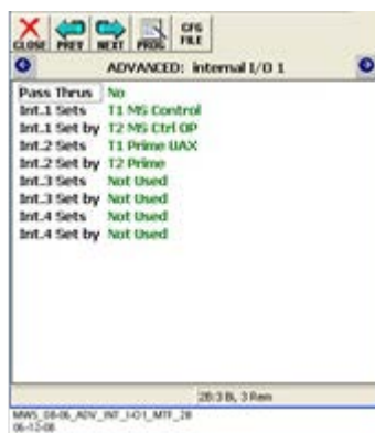
Figure 5-60: Crossing A Track 1 Internal I/O Programming Assignment
