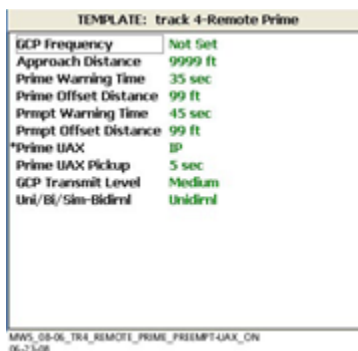
Figure 10-15: TEMPLATE: Track “N”- Remote Prime Window with Preemption set to “Advnce” and Prime UAX set to On
