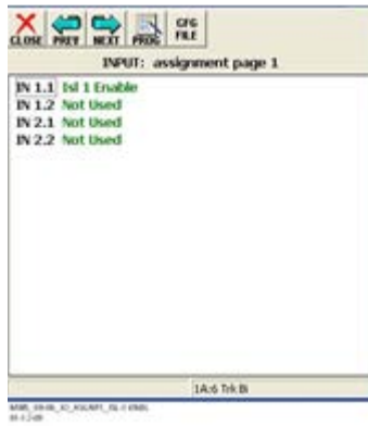
Figure 5-31: Input Assignment For External Island Configuration
