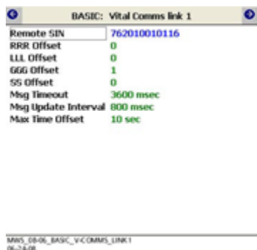
Figure 10-40: BASIC: Vital Comms link 1 Window
