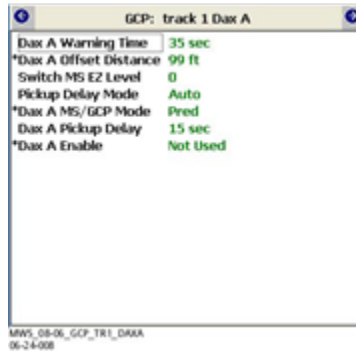
Figure 10-49: GCP: Track “N” Dax A Window
