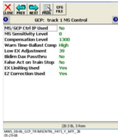
Figure 6-136: Bidirectional DAX Passthru Parameter
