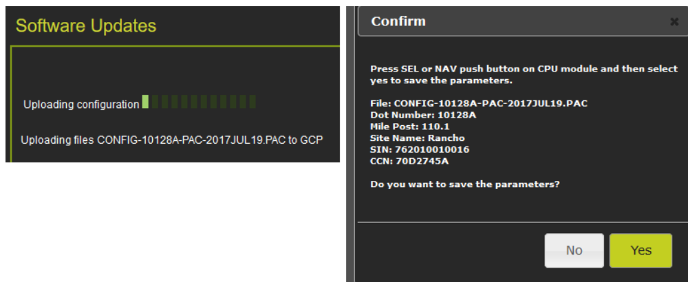
Figure 4-113 WebUI: Configuration Upload Progress and Final Check
