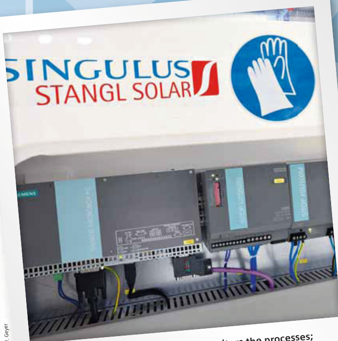
A Simatic Microbox PC controls and monitors the processes; Sitop power supply units provide for a reliable power supply
